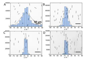
Fig. 4 Histograms and distributions of the orientation angle  $\alpha$  at different flow rates (A: 2.5 mL  $h^{-1}$ , B: 5 mL  $h^{-1}$ , C: 10 mL  $h^{-1}$ , D: 20 mL  $h^{-1}$ ). The background shows an exemplary video snapshot (xy-plane) with the respective flow rate (flow going from left to right)
