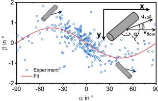
Fig. 3 Relation between the rod orientation angle  $\alpha$  and the angle of motion direction  $\beta$  at a flow rate of 2.5 mL h<sup>-1</sup> with a fit using eqn (1). The definition of  $\alpha$  and  $\beta$  is shown in the inset.
