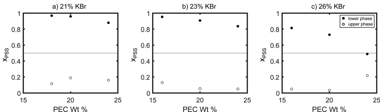
Fig. 6 Mole fraction of PSS in the dense (filled circles) and dilute (open circles) phases of samples prepared with (a) 21%, (b) 23%, and (c) 26% KBr by weight. The dashed line at  $x_{\text{PSS}} = 0.5$  indicates the composition of a stoichiometrically-balanced mixture.
