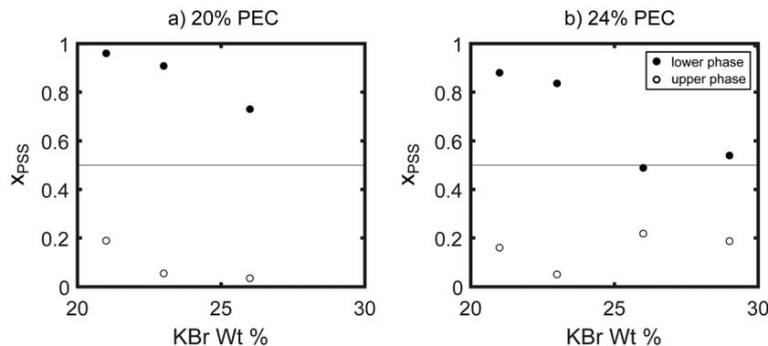
Fig. 7 Mole fraction of PSS in the dense (filled circles) and dilute (open circles) phases of samples prepared with (a) 20% and (b) 24% PEC by weight. The dashed line at  $\chi_{\text{PSS}} = 0.5$  indicates the composition of a stoichiometrically-balanced mixture.
