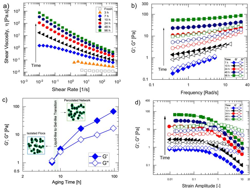
Fig. 1 (a) Steady-shear rheology, (b) frequency sweep, (c) summary of moduli at  $5.18 \text{ rad s}^{-1}$  from the frequency sweep data and (d) amplitude sweep data at different aging times of water-rich inks (20%  $\text{IrO}_2$ –0.2 l/C–90%  $\text{H}_2\text{O}$  in dispersion medium). The lines in plots (c) are only a guide-to-eye.
