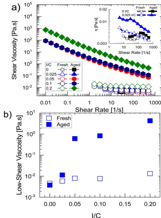
Fig. 3 (a) Steady-shear rheology of fresh and aged (96 h) inks as function of I/C consisting of 20% IrO<sub>2</sub> and 90% H<sub>2</sub>O in the medium. (b) Low-shear viscosity (~10 s<sup>-1</sup>) comparison between fresh and aged water-rich inks (90% H<sub>2</sub>O) as a function of I/C. The inset in figure a shows zoomed-in data of fresh inks.
