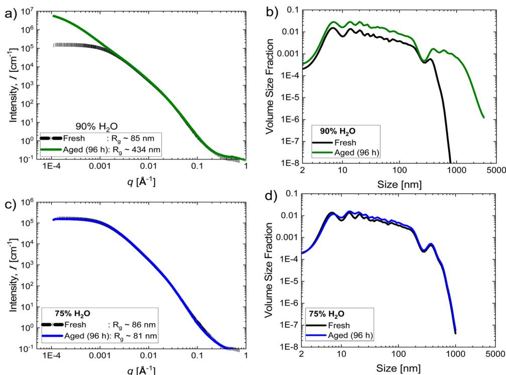
Fig. 2 (a) and (c) Scattering curves – intensity versus scattering vector  $q$  – and (b) and (d) volume size distribution of fresh and aged inks (96 h aging time) in (a) and (b) 90%  $\text{H}_2\text{O}$  and (c) and (d) 75%  $\text{H}_2\text{O}$  dispersion media at 20%  $\text{IrO}_2$  and 0.2 I/C.
