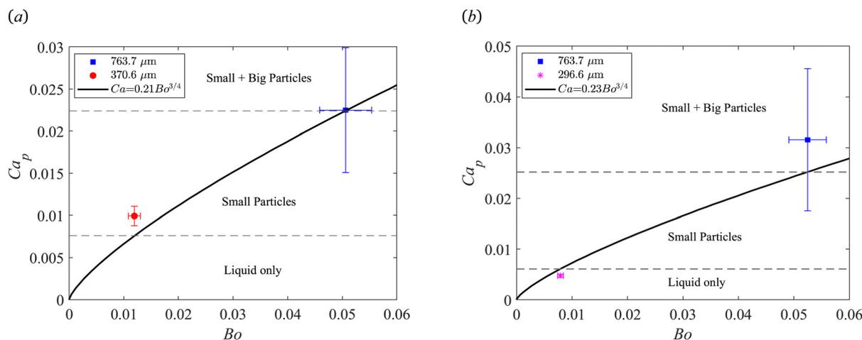
Fig. 9 Particle sorting of bidisperse suspensions. Capillary number  $Ca_p$  against bond number  $Bo$  for particle diameters (a)  $2a = 763.7 \mu\text{m}$  and  $2a = 370.6 \mu\text{m}$ , and (b)  $2a = 763.7 \mu\text{m}$  and  $2a = 296.6 \mu\text{m}$ . The dashed lines bound the active filtration region predicted by eqn (18). The solid lines indicate the predicted entrainment threshold from eqn (18) for (a)  $D = 0.21$  and (b)  $D = 0.23$ .
