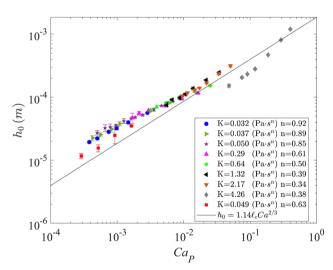
Fig. 4 Coating thickness  $h_0$  against capillary number  $Ca_p$  for solutions 1-9 in Table 2. The data are fit to the Landau-Levich-Derjaguin (LLD) law with a prefactor D = 1.14 (solid line).
