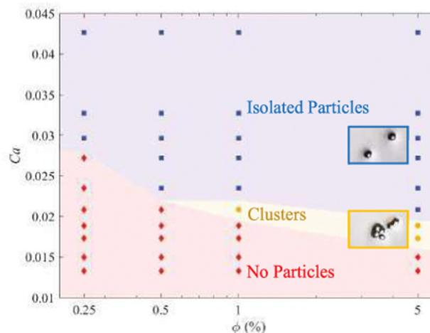
Fig. 5 Phase diagram ( $\phi$ ,  $Ca_p$ ) of the three monodisperse entrainment regimes showing no particles (red diamonds), clusters (yellow circles), and isolated particles (blue squares). Data markers correspond to experiments with fixed particle diameter  $2a = 763.7 \mu\text{m}$ .
