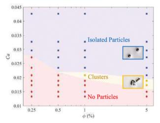
Fig. 5 Phase diagram ( $\phi$ , Ca<sub>p</sub>) of the three monodisperse entrainment regimes showing no particles (red diamonds), clusters (yellow circles), and isolated particles (blue squares). Data markers correspond to experiments with fixed particle diameter  $2a = 763.7 \mu m$ .
