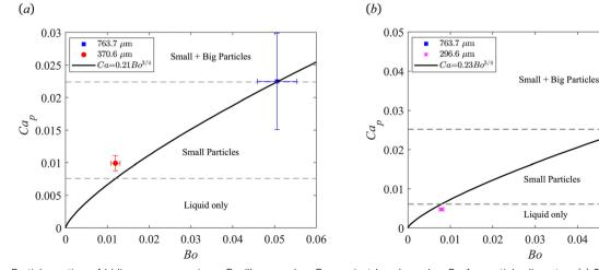
Fig. 9 Particle sorting of bidisperse suspensions. Capillary number  $Ca_p$  against bond number Bo for particle diameters (a)  $2a = 763.7 \mu m$  and  $2a = 763.7 \mu m$  and 2a = 763 $370.6 \, \mu m$ , and (b)  $2a = 763.7 \, \mu m$  and  $2a = 296.6 \, \mu m$ . The dashed lines bound the active filtration region predicted by eqn (18). The solid lines indicate the predicted entrainment threshold from eqn (18) for (a) D = 0.21 and (b) D = 0.23.
