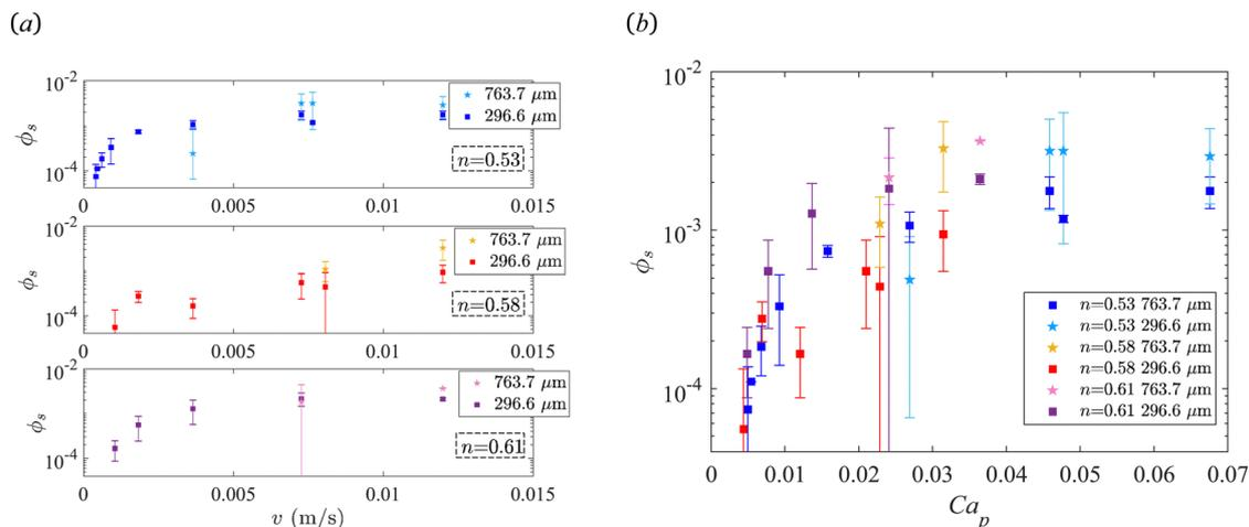
Fig. 8 Surface coverage  $\phi_s$  of entrained particles against (a) the withdrawal velocity  $v$  and (b) the capillary number  $Ca_p$  for three bidisperse solutions with particle sizes  $2a = 763.7 \mu\text{m}$  and  $2a = 296.6 \mu\text{m}$  and power-law index  $n = 0.53, 0.58,$  and  $0.61$ .
