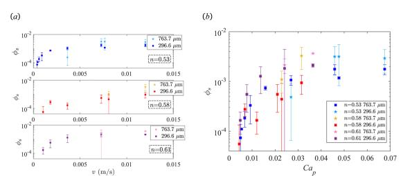
Fig. 8 Surface coverage  $\phi_s$  of entrained particles against (a) the withdrawl velocity v and (b) the capillary number Ca<sub>D</sub> for three bidisperse solutions with particle sizes  $2a = 763.7 \, \mu m$  and  $2a = 296.6 \, \mu m$  and power-law index n = 0.53, 0.58, and 0.61.
