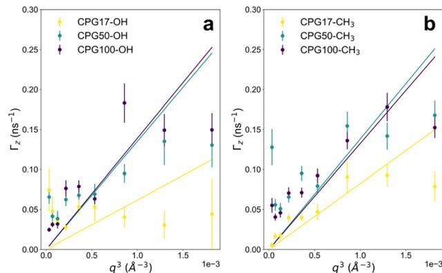
**Fig. 7** Relaxation rate  $\Gamma_z$  obtained from fitting eqn (7) in dependence on  $q^3$  of the microemulsion confined in hydrophilic (a) and hydrophobic CPG (b).
