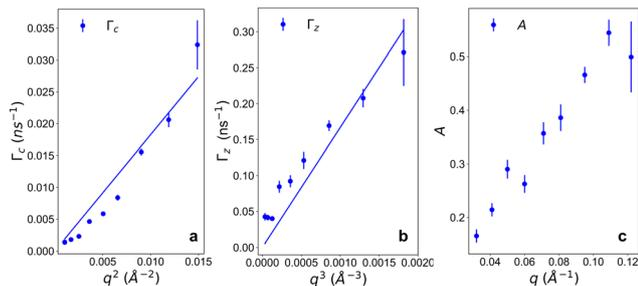
Fig. 4 Results of fitting the NSE data of Fig. 3(a) with eqn (7): (a) relaxation rate  $\Gamma_c$  of the collective motions inside the bicontinuous microemulsions (b) relaxation rate  $\Gamma_z$  of the membrane undulations and (c) amplitude  $A$  as a measure of the weight of the contribution of both dynamics.
