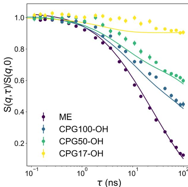
Fig. 5 Normalized intermediate scattering function of the bicontinuous microemulsion in bulk (ME) and confined in CPG100-OH, CPG50-OH, CPG17-OH at  $q = 0.095 \text{ \AA}^{-1}$  with the fit to the eqn (9).
