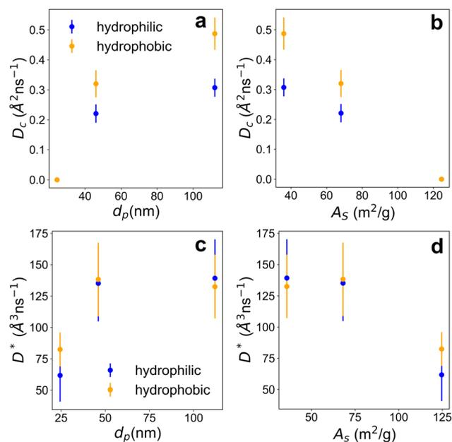
**Fig. 8** The diffusion coefficient  $D_c$  in dependence of the pore diameter  $d_p$  (a) and the specific surface area  $A_s$  (b).  $D^*$  plotted against the pore diameter  $d_p$  (c) and the specific surface area  $A_s$  (d). The blue data points are for the confined microemulsion in hydrophilic pores and yellow for hydrophobic pores.
