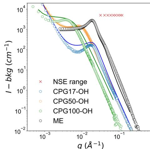
Fig. 2 SANS signal of the hydrophilic D<sub>2</sub>O-filled CPG and the bicontinuous microemulsion in bulk (ME). The solid line represents the fit to the eqn (2). The red crosses represent the investigated  $q$ -range by NSE.
