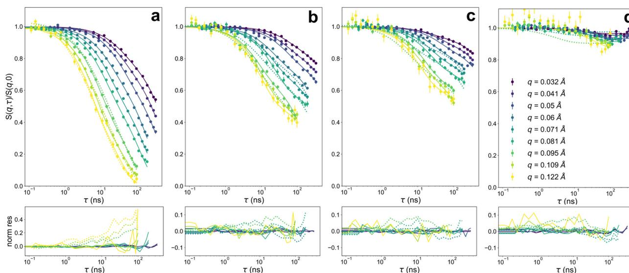
Fig. 3 Normalized intermediate scattering functions of (a) the bicontinuous microemulsion in bulk and the confined microemulsion in the hydrophilic CPG100-OH (b), CPG50-OH (c) and CPG17-OH (d) for several  $q$  values. The solid lines are fits to the eqn (7). The dotted lines are the fit to the eqn (9). Bottom: Normalized residuals of the fit.
