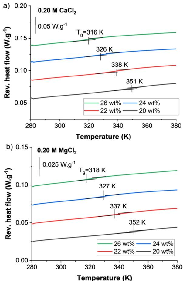
Fig. 3 MDSC Reversing heat flow curves for PDADMA–PSS PECs showing the glass transition from the second heating cycle for (a) 0.20 M  $\text{CaCl}_2$  and (b) 0.20 M  $\text{MgCl}_2$  PECs at varying water content (20–26 wt% added water). Curves shifted across the y-axis by a 20% gap for clarity. Exotherm down.
