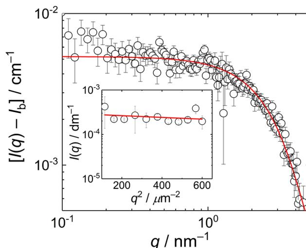
Fig. 1 SANS curve of  $10 \text{ mg mL}^{-1}$  MFC solution, rear detector distance 5.6 m. Inset: Guinier plot of the static light scattering data from  $10 \text{ mg mL}^{-1}$  MFC solution. The red lines are the fits of the data with the Guinier equation.
