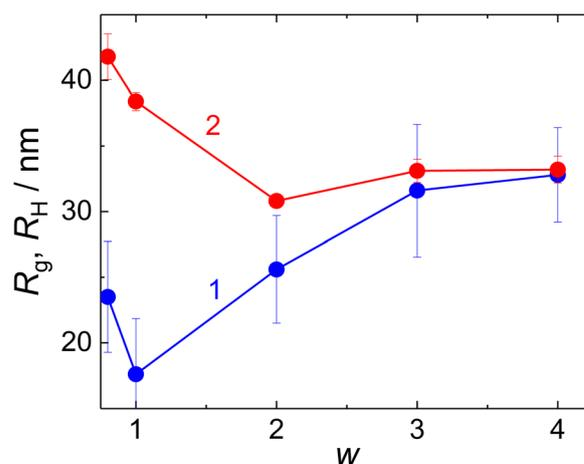
Fig. 4 Gyration radius,  $R_g$  (curve 1), and hydrodynamic radius,  $R_H$  (curve 2) of MFC/PMAA-PEO particles, as functions of  $w$ .
