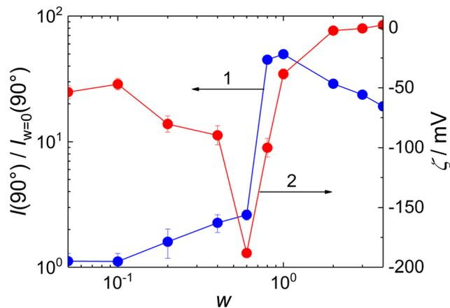
Fig. 5 Right-angle scattering intensity  $I(90^\circ)$  (curve 1), relatively to forward scattering intensity at  $w = 0$ ,  $I(90^\circ)_{w=0}$  and zeta potential (curve 2) for static light scattering of MFC/PMAA-PEO mixtures as functions of MFC-to-PMAA-PEO mass ratios,  $w$ .
