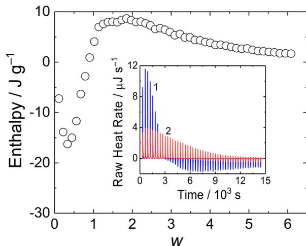
Fig. 8 Enthalpy curve for titration of MFC into PMAA-PEO solution plotted against MFC to PMAA-PEO mass ratio,  $w$ . Inset: ITC raw data for titration of MFC into PMAA-PEO solution (curve 1) and into CAPSO buffer (curve 2).
