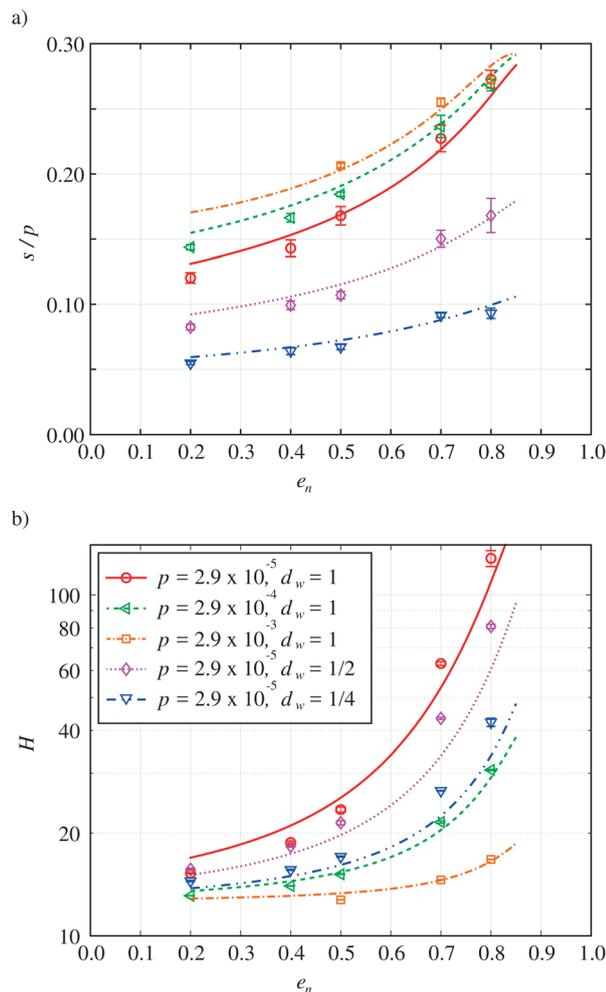
**Fig. 9** Measured (symbols) and predicted (lines) (a) macroscopic friction and (b) flow height as functions of the coefficient of restitution for  $h = 7.94$  and:  $d_w = 1$  and  $p = 2.9 \times 10^{-5}$  (red circles);  $d_w = 1$  and  $p = 2.9 \times 10^{-4}$  (green triangles);  $d_w = 1$  and  $p = 2.9 \times 10^{-3}$  (orange squares);  $d_w = 1/2$  and  $p = 2.9 \times 10^{-5}$  (purple diamonds);  $d_w = 1/4$  and  $p = 2.9 \times 10^{-5}$  (blue lower triangles).
