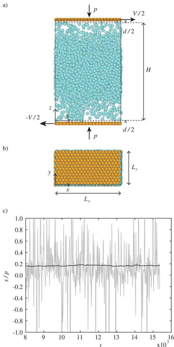
**Fig. 1** (a) Snapshot of a typical pressure-imposed simulation once the steady state is attained. Also shown is the frame of reference. (b) Top view of the bumpy plane composed of regularly arranged spheres. (c) Temporal evolution of the instantaneous (light grey line) and the smoothed (black line) stress ratio for a typical simulation in steady state ( $p = 2.9 \times 10^{-5}$ ,  $d_w = 1$  and  $e_n = 0.5$ ).
