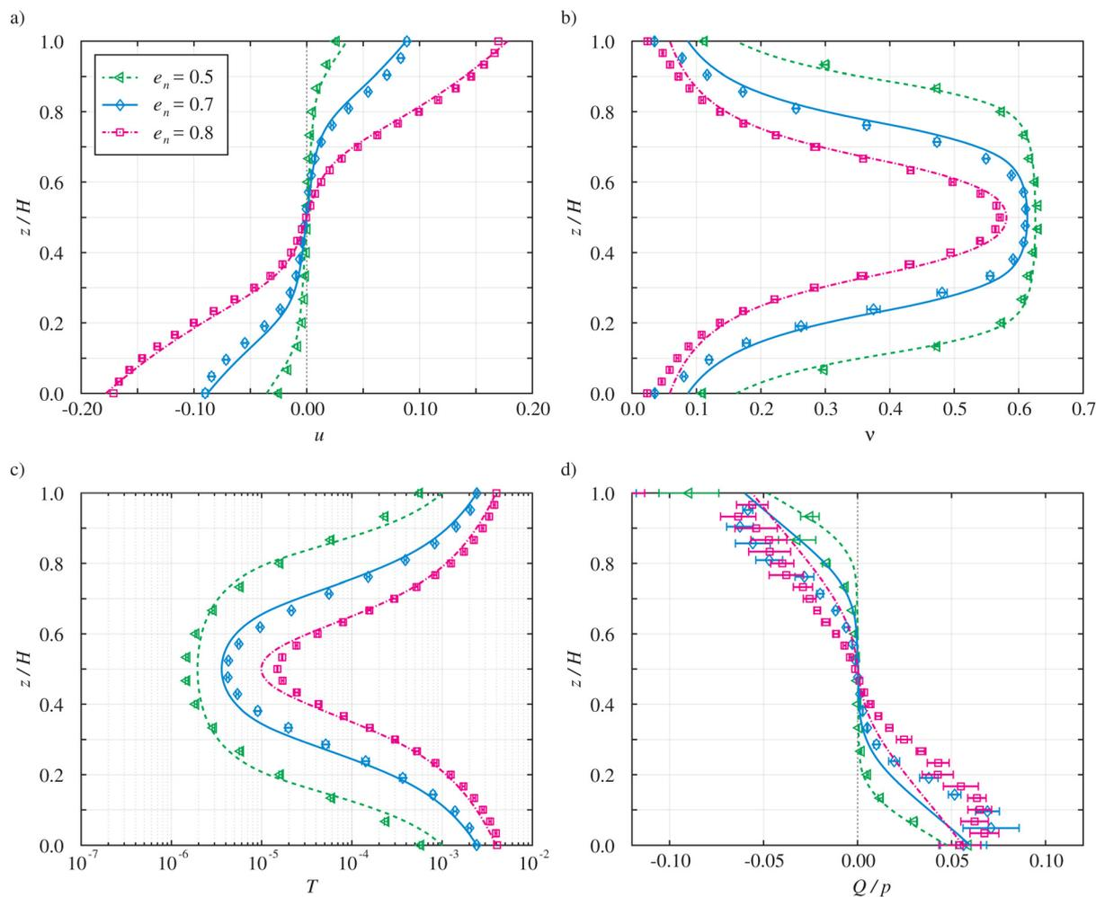
Fig. 5 Measured (symbols) and predicted (lines) profiles of (a) mean velocity, (b) solid volume fraction, (c) granular temperature and (d) normalized fluctuation energy flux,  $Q/p$ , for  $p = 2.9 \times 10^{-4}$ ,  $d_w = 1$ ,  $h = 7.94$ , and different values of the coefficient of restitution  $e_n$  (see the legend in (a)).
