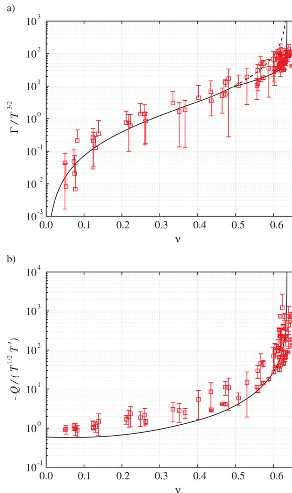
Fig. 3 Measurements in DEM simulations (symbols) against predictions of kinetic theory (eqn (4) and (5), lines) of (a) the scaled rate of collisional dissipation and (b) the scaled diffusivity as functions of the solid volume fraction, for  $e_n = 0.5$ . The solid and dashed lines in (a) are eqn (4) when the correlation length  $L$  is given by eqn (7) and when  $L = 1$ , respectively.
