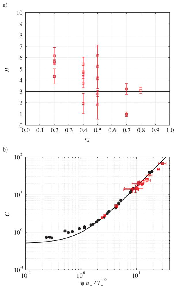
Fig. 4 Coefficients (a)  $B$  as a function of the coefficient of restitution and (b)  $C$  as a function of the scaled slip velocity, measured in DEM simulations of pressure-imposed (open squares) and volume-imposed (filled circles, after ref. 25) shearing flows between rigid, bumpy planes. Also shown are the expressions  $B = 3$  and eqn (20) (solid lines).
