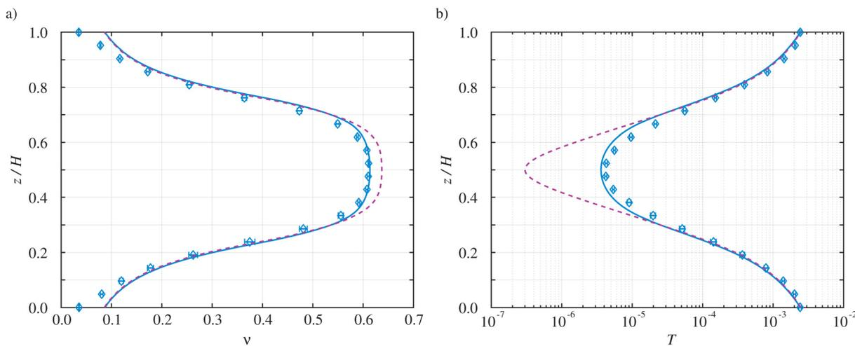
Fig. 6 Profiles of (a) solid volume fraction and (b) granular temperature predicted by the theory when the correlation length is given by eqn (6) (solid lines) and  $L = 1$  (dashed lines), for the case  $p = 2.9 \times 10^{-4}$ ,  $d_w = 1$  and  $e_n = 0.7$ . Also plotted are the numerical measurements obtained in the simulation (symbols).
