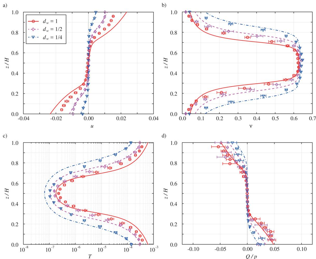
Fig. 8 Measured (symbols) and predicted (lines) profiles of (a) mean velocity, (b) solid volume fraction, (c) granular temperature and (d) normalized fluctuation energy flux,  $Q/p$ , for  $e_n = 0.5$ ,  $p = 2.9 \times 10^{-5}$ ,  $h = 7.94$ , and different values of the boundary particle diameter  $d_w$  (see the legend in (a)).
