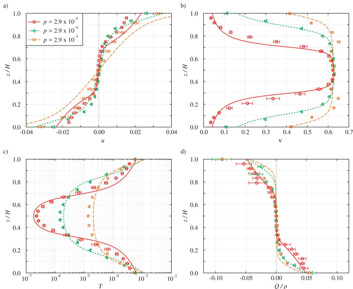
Fig. 7 Measured (symbols) and predicted (lines) profiles of (a) mean velocity, (b) solid volume fraction, (c) granular temperature and (d) normalized fluctuation energy flux,  $Q/p$ , for  $e_n = 0.5$ ,  $d_w = 1$ ,  $h = 7.94$ , and different values of the imposed pressure  $p$  (see the legend in (a)).
