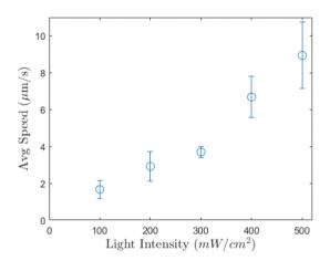
Fig. 2 The average speed of the larger TiO<sub>2</sub> micromotors as a function of light intensity at a hydrogen peroxide concentration of 15%. Error bars represent standard error of the mean
