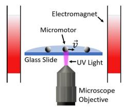
Fig. 1 A schematic of the experimental setup
