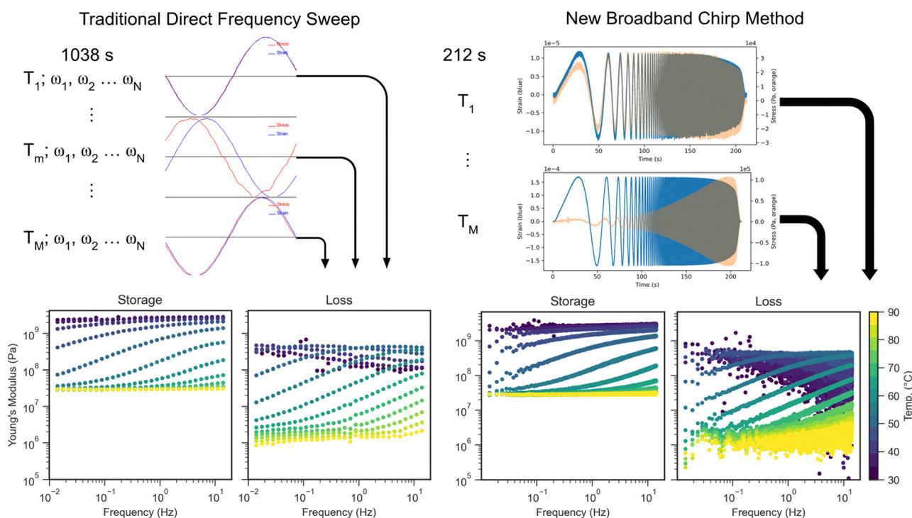
**Fig. 2** Comparison of log-spaced direct frequency sweep (DFS) (left) and broadband chirp (right) approaches to temperature-dependent modulus measurement. While the storage and loss moduli match between approaches in terms of magnitude and frequency trend at each  $T_M$ , data density and variance differ.
