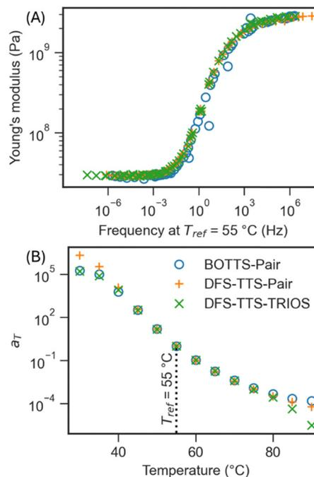
Fig. 6 (A) Storage modulus curves and (B) horizontal shift factors for master curves from pairwise BOTTs (blue circles), pairwise DFS-TTS (orange plus), and DFS-TTS derived from the commercial TRIOS software. The reference temperature 55 °C is indicated by a dashed line.
