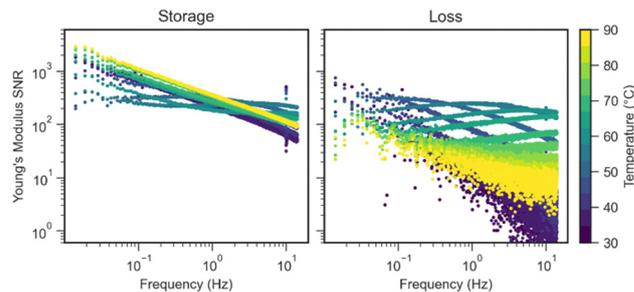
Fig. 3 Complex Young's modulus magnitude over the propagated error, *i.e.*, "Signal-to-Noise Ratio" (SNR) for chirps on PT resin at each temperature.
