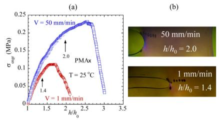
Fig. 4 (a) Engineering stress vs. stretching ratio curves from pure shear stretching of PMA specimens at crosshead speeds V = 1 and 50 mm min<sup>-1</sup>. (b) Images of the notch tip at onset of fracture described in (a).
