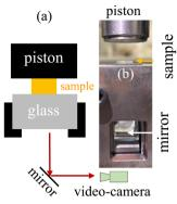
Fig. 1 (a) Schematic illustration of the compression setup for video recording. (b) Photo of the actual setup. Piston is mounted on the moving crosshead of the Instron.
