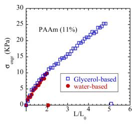
Fig. 8 Engineering stress vs. nominal stretching ratio from uniaxial extension of dogbone-shaped water-based and glycerol-based polyacrylamide specimens at constant crosshead velocity of 1 mm s<sup>-1</sup>. Both specimens have the same dimensions: L = 26 mm, w = 2.8 mm, t = 2.6 mm.
