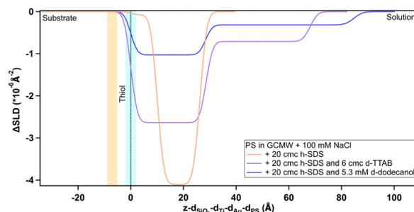
Fig. 10 Depth profile, after subtraction of the substrate profile, of adsorbed species on PS as indicated on the graph. The blue panel, centred at the dotted line at  $x = 0$ , and the yellow panel on its left indicate, respectively, the PS/adsorbed layer and Au/PS interfaces with their associated roughness. The profile in the case of 20 cmc h-SDS is the same curve of Fig. 9.
