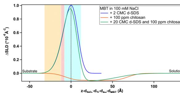
Fig. 12 Depth profile, after subtraction of the substrate profile, of adsorbed species on MBT as indicated on the graph. The blue panel, centred at the dotted line at  $x = 0$ , indicates the MBT/adsorbed layer interface. The yellow panel indicates the Au/MBT interface. The widths are due to roughness, which causes an overlapping (striped area).
