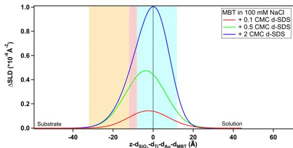
Fig. 7 Depth profile, after subtraction of the substrate profile, of d-SDS adsorbed on MBT (bulk d-SDS concentrations indicated in the figure). The blue panel, centred at the dotted line at  $x = 0$ , indicates the MBT/d-SDS interface. The yellow panel indicates the Au/MBT interface. The widths are due to roughness, which causes an overlapping (striped area).
