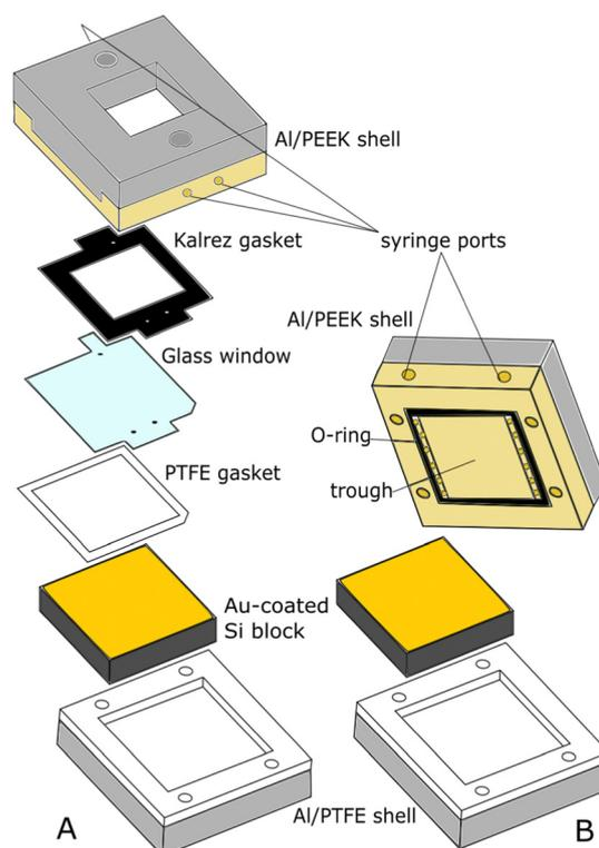
Fig. 2 Expanded view of the solid/liquid cells used in the NR experiments. (A) “Custom”  $65 \times 65 \text{ mm}^2$  cell. The liquid phase is injected through the ports in the PEEK shell and contained in the trough formed by the PTFE gasket between the gold surface and the glass window; (B) “typical”  $50 \times 50 \text{ mm}^2$  cell, where the trough is in the PEEK shell, sealed by a O-ring.
