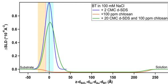
Fig. 13 Depth profile, after subtraction of the substrate profile, of adsorbed species on BT as indicated on the graph. The blue panel, centred at the dotted line at  $x = 0$ , indicates the BT/d-SDS interface. The yellow panel indicates the Au/BT interface. The widths are due to roughness, which causes an overlapping (striped area).
