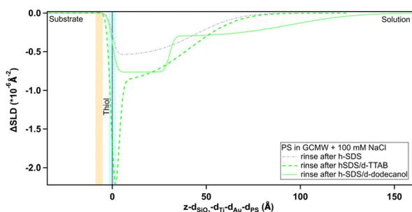
Fig. 15 Depth profile, after subtraction of the substrate profile, of residual adsorbed species on PS after the rinses indicated on the graph. The blue panel, centred at the dotted line at  $x = 0$ , and the yellow panel on its left indicate, respectively, the PS/adsorbed layer and Au/PS interfaces with their associated roughness.
