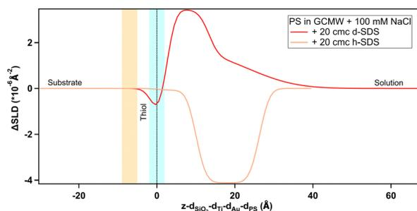
Fig. 9 Depth profile, after subtraction of the substrate profile, of adsorbed SDS on PS (deuteration and concentration indicated on the graph). The blue panel, centred at the dotted line at  $x = 0$ , and the yellow panel on its left indicate, respectively, the PS/d-SDS and Au/PS interfaces with their associated roughness.
