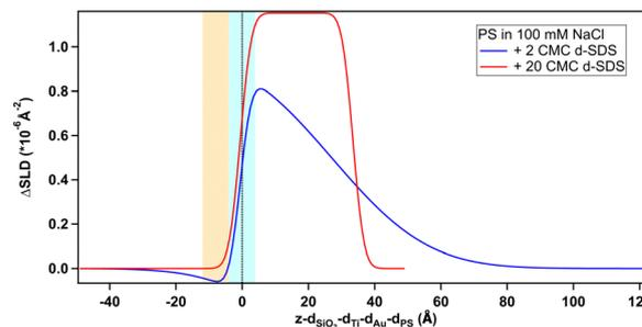
Fig. 8 Depth profile, after subtraction of the substrate profile, of d-SDS adsorbed on PS (bulk d-SDS concentrations indicated in the figure). The blue panel, centred at the dotted line at  $x = 0$ , and the yellow panel on its left indicate, respectively, the PS/d-SDS and Au/PS interfaces with their associated roughness.
