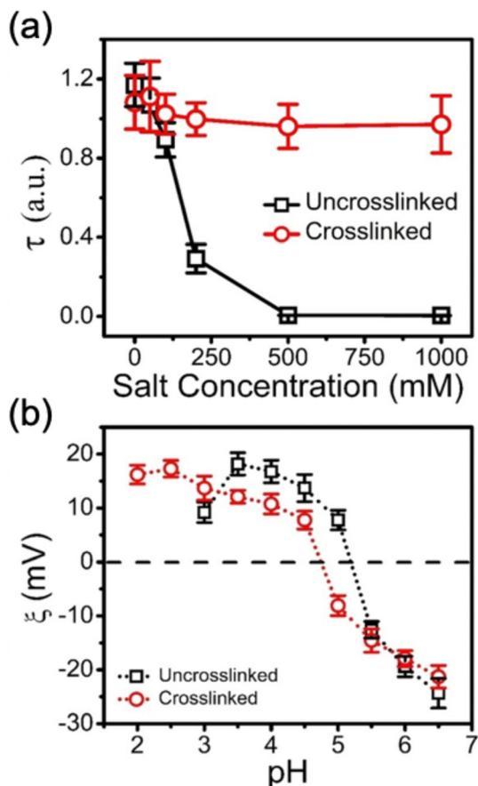
Fig. 2 (a) Turbidity of uncrosslinked ( $\square$ ) and crosslinked ( $\circ$ ) BPEI-allyl-PAA coacervate droplets as a function of increasing NaCl concentration from 0 to 1000 mM. (b) Zeta potential of BPEI-allyl-PAA coacervates as a function of pH. Error bars represent the standard deviations of the three measurements.
