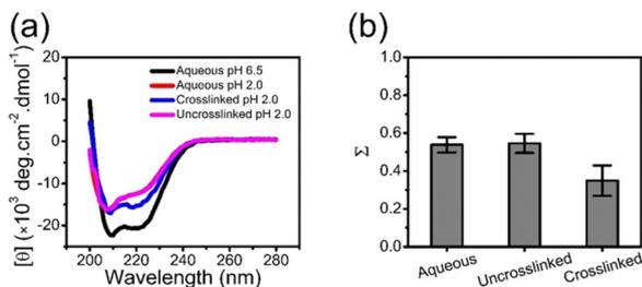
**Fig. 6** (a) CD spectra of BSA in aqueous solution at pH 6.5 (black) and 2.0 (red), and in uncrosslinked (magenta) and crosslinked (blue) coacervates at pH 2.0. (b) Fraction of unfolded BSA at pH 2.0, in aqueous solution, and in uncrosslinked and crosslinked coacervates. The error bars represent the standard deviation of the 3 measurements.
