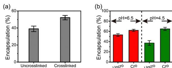
Fig. 4 (a) BSA encapsulation efficiency of uncrosslinked and crosslinked coacervates at pH 6.5, and (b) ALP encapsulation efficiency of uncrosslinked (Uncro) and crosslinked (Cro) coacervates at pH 6.5 and 4.5. The error bars represent the standard deviations of the three measurements.
