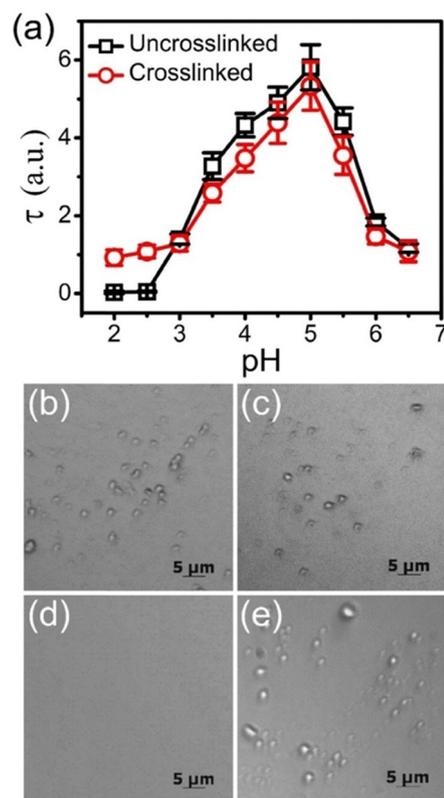
Fig. 1 (a) Turbidity of uncrosslinked ( $\square$ ) and crosslinked ( $\circ$ ) BPEI-allyl-PAA coacervate droplets as a function of decreasing pH from 6.5 to 2.0. Optical micrographs of (b) uncrosslinked and (c) crosslinked coacervate droplets at pH 6.5 as well as (d) uncrosslinked and (e) crosslinked coacervate droplets at pH 2.0. Error bars represent the standard deviations from three measurements.
