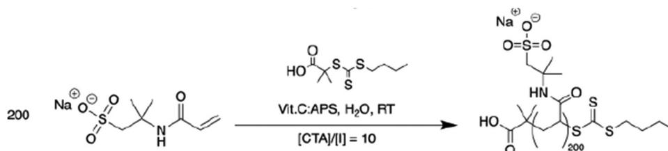
Scheme 2 Redox-RAFT polymerization leading to anionic macroCTA.
