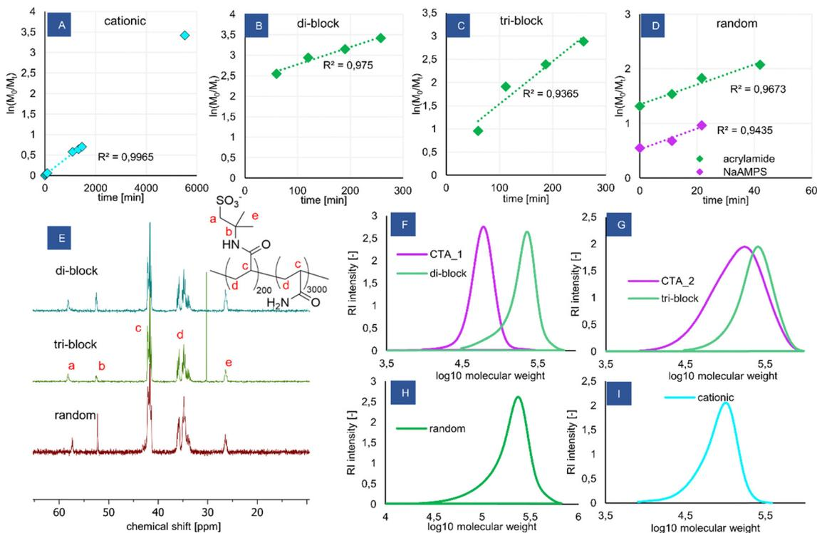
Fig. 1 Synthesis of the copolymers and analysis of the products. (A)–(D) Kinetic plots for the polymerization reactions determined using  $^1\text{H}$  NMR, (E) quantitative  $^{13}\text{C}$  NMR spectra of the products recorded in  $\text{D}_2\text{O}$  with an inverse-gated decoupling pulse sequence, (F)–(I) molecular weight distributions determined using aqueous SEC.
