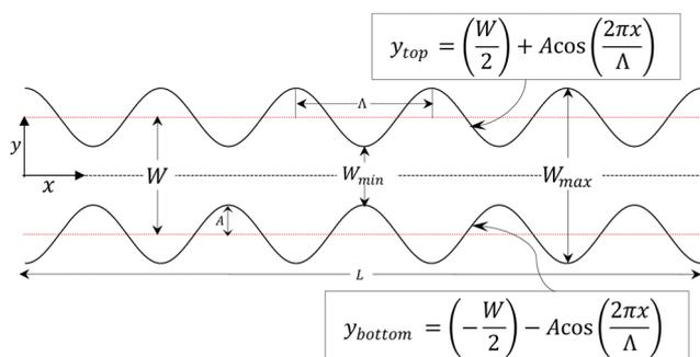
**Fig. 1** Schematic diagram of the corrugated channel used in the simulations:  $A$  and  $\Lambda$  are the amplitude and wavelength of the corrugations, respectively,  $L$  is the length,  $W$  is the mean width,  $W_{\text{min}}$  is the minimum width and  $W_{\text{max}}$  is the maximum width of the channel. The boxed equations in the figure describe the geometry of the top and bottom wall of the channel.
