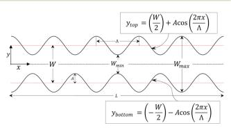
Fig. 1 Schematic diagram of the corrugated channel used in the simulations: A and  $\Lambda$  are the amplitude and wavelength of the corrugations, respectively, L is the length, W is the mean width,  $W_{\min}$  is the minimum width and  $W_{\rm max}$  is the maximum width of the channel. The boxed equations in the figure describe the geometry of the top and bottom wall of the channel.
