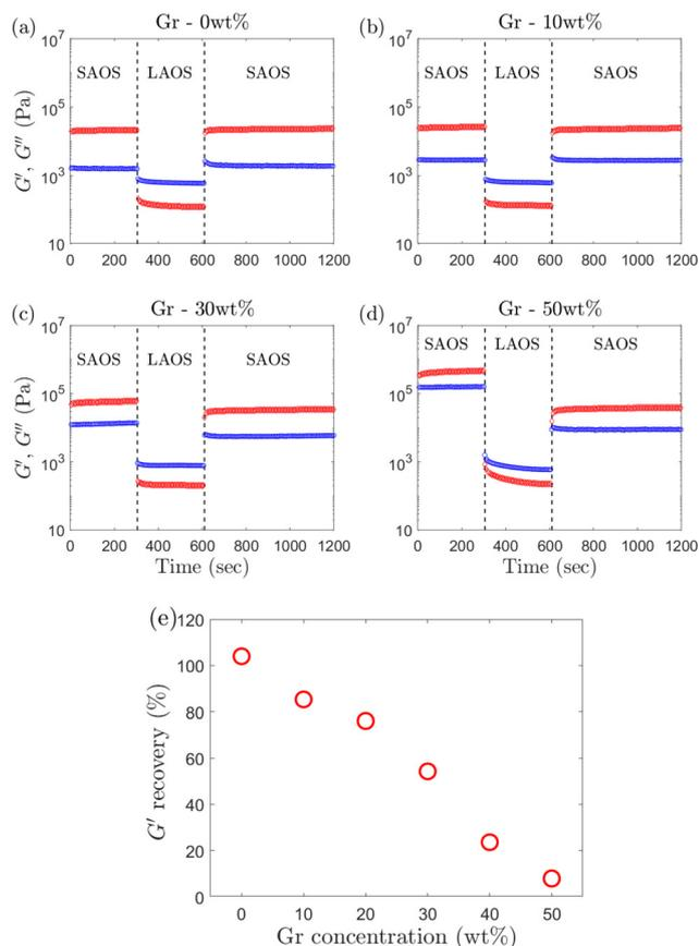
**Fig. 10** Recovery of  $G'$  (red symbol) and  $G''$  (blue symbol) with varying Gr concentrations, (a) 0 wt%, (b) 10 wt%, (c) 30 wt%, and (d) 50 wt%. (e) Recovery of  $G'$  after the LAOS step with varying Gr concentrations. The  $G'$  value, 200 seconds after the start of recovery (called as  $G'_{\text{rec}}$ ), is considered for the calculation, in order to avoid any major transient phenomenon (which exists until around  $\approx 100$  seconds as can be seen in Fig. 11(a)).
