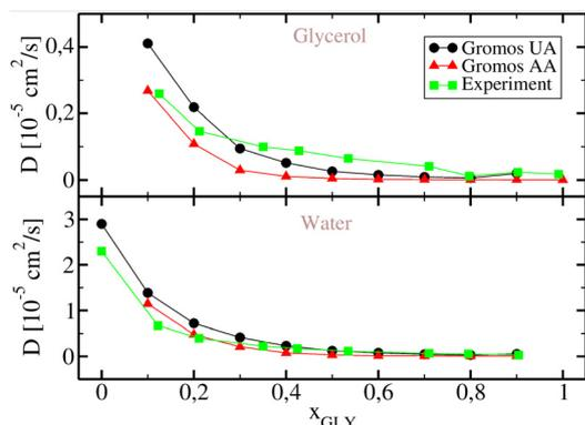
Fig. 8 Self-diffusion coefficients of glycerol (top panel) and water (bottom panel) versus glycerol mole fraction  $x_{\text{GLY}}$ . Black dots are for the UA model, red triangles are for the AA model and green squares are for experimental data.
