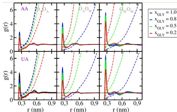
Fig. 4 O–O RDFs and running coordination numbers for all-atom (AA) and united-atom (UA) force fields. Left panels:  $O_A-O_A$ , middle panels:  $O_A-O_W$ , right panels:  $O_W-O_W$ . Color convention:  $x_{GLY} = 1.0$  (black),  $x_{GLY} = 0.8$  (blue),  $x_{GLY} = 0.5$  (green) and  $x_{GLY} = 0.2$  (red).
