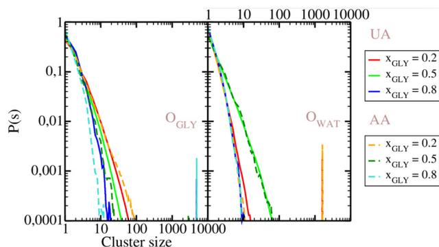
Fig. 6 Cluster distribution functions for OO atoms of glycerol (left panel) and water (right panel). Full lines, UA model:  $x_{GLY} = 0.2$  (red),  $x_{GLY} = 0.5$  (green),  $x_{GLY} = 0.8$  (blue). Dashed lines, AA model:  $x_{GLY} = 0.2$  (orange),  $x_{GLY} = 0.5$  (dark green),  $x_{GLY} = 0.8$  (cyan).
