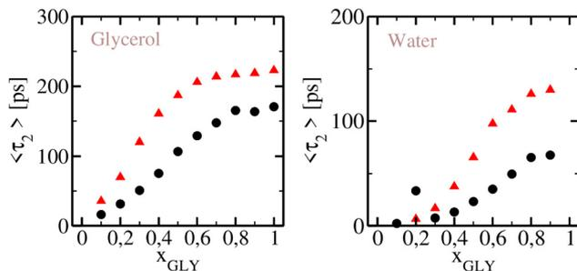
Fig. 11 Integral correlation times  $\langle \tau_2 \rangle$  for glycerol (left panel) and water (right panel). Black dots are results for the UA glycerol mixture and red triangles are for the AA glycerol mixture.
