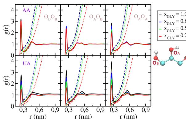
Fig. 3  $O_{\text{GLY}}$ – $O_{\text{GLY}}$  RDFs and running coordination numbers for all-atom (AA) and united-atom (UA) force fields. Pictorial representation of the molecule is seen on the left with tags indicating two oxygen sites in glycerol. Left panels:  $O_B$ – $O_B$ , middle panels:  $O_A$ – $O_B$ , right panels:  $O_A$ – $O_A$ . Color convention:  $x_{\text{GLY}} = 1.0$  (black),  $x_{\text{GLY}} = 0.8$  (blue),  $x_{\text{GLY}} = 0.5$  (green) and  $x_{\text{GLY}} = 0.2$  (red).
