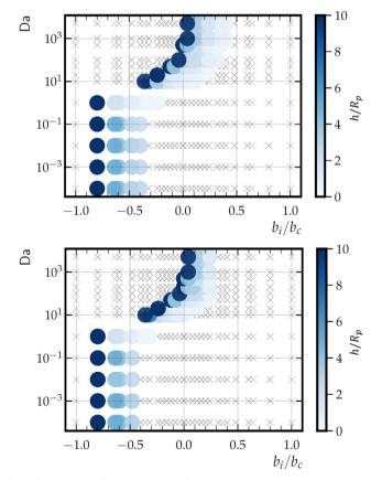
Fig. 13 Hovering "phase diagrams" for a cap-up sphere near a circular patch with radius  $R_d$  = 1/3 (above) and  $R_d$  = 3 (below). The diagrams illustrate the existence (symbols) and location (colour code) of hovering states as a function of the parameters Da and  $b_i/b_c$ . The phase diagrams are restricted to hovering states with  $1 \le h/R_p \le 10$ .
