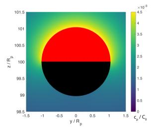
Fig. 4 Concentration of the chemical product for a cap-up sphere located far away from the wall  $(h/R_p = 100)$  with Da = 100. The concentration is mostly uniform over the cap, with a sharp drop as one approaches the "equator" from the catalytic pole (note that the yellow region is thinner near the equator.) This variation is in contrast with the "inversion" effect seen for Da = 100 in Fig. 3. The patch size is  $R_d = R_p$ , and the concentration was computed with the BEM
