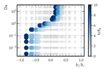
Fig. 12 Hovering "phase diagram" illustrating the existence (symbols) and location (colour code) of hovering states as a function of the parameters Da and  $b_i/b_c$ . The results correspond to a sphere in a cap-up orientation near a circular patch with  $R_d = R_p$ , and the phase diagram is restricted to hovering states with  $1 \le h/R_p \le 10$ .
