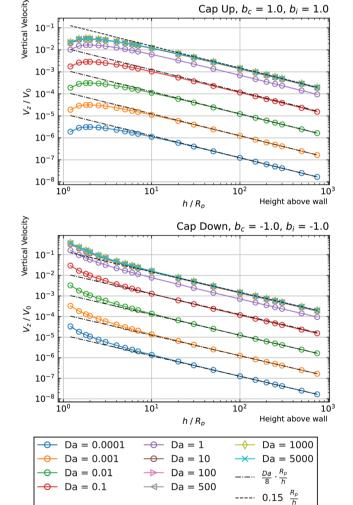
Fig. 5 Dependence of the vertical velocity  $V_z$  on the height h for a sphere with uniform surface mobility near a circular patch. Predicted low Da and high Da scalings are given by dotted-dashed and dashed lines, respectively. The sign of the surface mobility is chosen to give a positive velocity. The patch has the same radius as the particle  $(R_d/R_p=1)$ .
