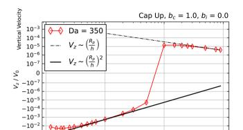
Fig. 8 Dependence of  $V_z$  on h for a cap-up sphere with  $b_c = 1$ ,  $b_i = 0$ , and Da = 350. Crossover between two power law scalings is clearly visible.
