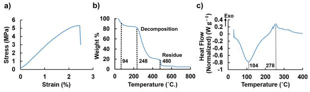
Fig. 2 (a) Representative stress-strain plot for tensile testing experiments with purified and cast promonan film. (b) Thermal decomposition of the material shown through thermogravimetric analysis for purified polysaccharide. (c) Analysis of the materials heat capacity tested using differential scanning calorimetry.
