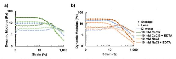
Fig. 4 (a) The addition of bivalent ions results in a significant increase in the dynamic moduli while the addition of EDTA chelates the ions (p-value < 0.01), reducing the dynamic moduli. (b) The addition of monovalent ions results in a small increase in dynamic moduli that cannot be reversed with EDTA, which does not chelate monovalent ions. These changes were not statistically significant (p-value > 0.01)
