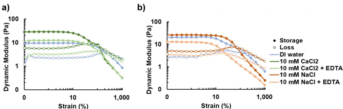
Fig. 4 (a) The addition of bivalent ions results in a significant increase in the dynamic moduli while the addition of EDTA chelates the ions ( $p$ -value < 0.01), reducing the dynamic moduli. (b) The addition of monovalent ions results in a small increase in dynamic moduli that cannot be reversed with EDTA, which does not chelate monovalent ions. These changes were not statistically significant ( $p$ -value > 0.01).
