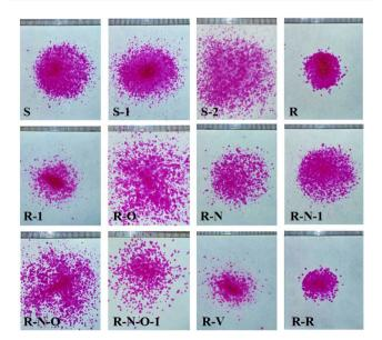
Fig. 4 Coating areas with different equipment configurations.
