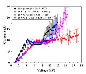
Fig. 9 Variation in currents with applied voltage for R-N, R-N-1, R-N-O, and R-N-O-1.
