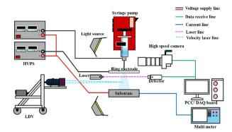
Fig. 1 Lab-scale experimental apparatus.
