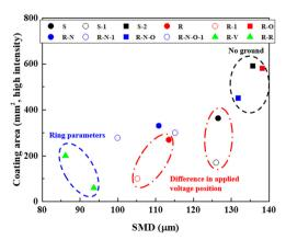
Fig. 11 High-intensity coating area as a function of SMD for different
