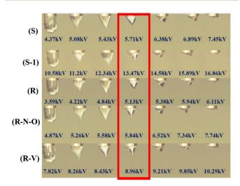
Fig. 3 Electrospray modes for different applied voltages.
