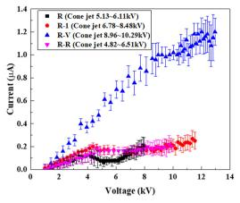
Fig. 8 Variation in current with applied voltage for R, R-1, R-V, and R-R.
