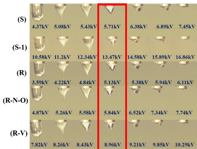
Fig. 3 Electro spray modes for different applied voltages.
