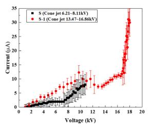
Fig. 7 Variation in current with applied voltage for S and S-1.
