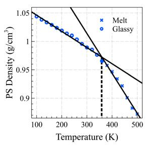
Fig. 1 The estimated glass transition temperature of the PS bulk is 358 K. determined by the intersection of the linear fits of density vs. temperature curves for the glassy and melt states.
