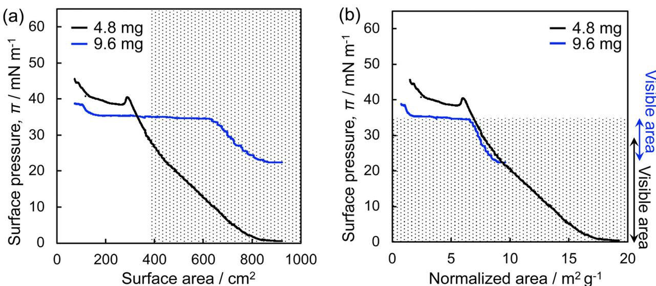
Fig. 3 (a) Surface pressure,  $\pi$ , versus surface area and (b) surface pressure versus normalized area (the interfacial area ( $\text{m}^2$ )/the amount of added microgel) compression isotherms for the microgels at the air/water interface. Different amounts of microgel (black: 4.8 mg; blue: 9.6 mg) were added. The dotted area shows the range in which the microgels can be visualized using fluorescence microscope during compression.
