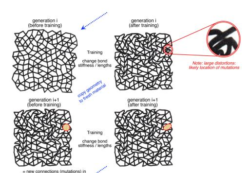
Fig. 2 Darwinian evolution with Larmarckian elements. Each generation of the material is physically trained and the next generation is made with fresh material in the geometry of the trained material. Mutations (change in topology) during the copying are likely in regions with particularly large distortion due to training. Images are of a laser-cut network (top left) that was then trained by compression (top right). These images were obtained from authors of ref 25
