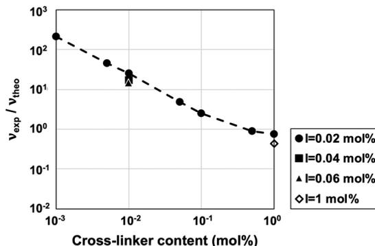
Fig. 3 Relationship between the cross-linker content in the pre-gel solution and the ratio of experimental to theoretical cross-linking densities ( $\nu_{\text{exp}}/\nu_{\text{theo}}$ ) of the ion gels.
