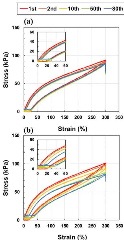
Fig. 5 Cyclic stress–strain curves at 300% strain at a tensile rate of  $10 \text{ cm min}^{-1}$  for the ion gels with cross-linker contents of (a) 0.01 mol% and (b) 0 mol% at the same initiator content of 0.02 mol%. Each cycle was separated by a waiting time of 600 s. The inset shows magnified images.
