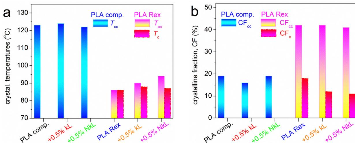
Fig. 5 DSC values of interest related to PLA's crystallization, in particular, (a)  $T_{cc}$  and  $T_c$  from scan 1 and scan 2, respectively, and (b)  $CF_{cc}$  and  $CF_c$  from scan 1 and scan 2, respectively.
