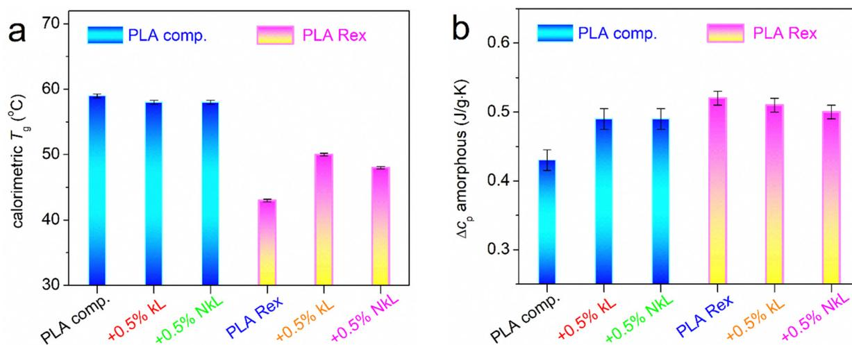
Fig. 4 Values related to the glass transition of PLA in the amorphous state (scan 1), in particular, (a)  $T_g$  and (b)  $\Delta c_p$ , shown in the form of column diagrams for all samples (description on the horizontal scale axis).
