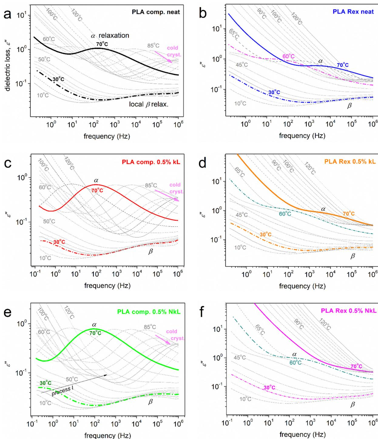
Fig. 7 BDS isothermal spectra in the form of frequency dependence of  $\epsilon''(f)$  in the overall range of temperature studied. The various dipolar processes recorded (local  $\beta$  and segmental  $\alpha$ ) are indicated on selected curves.
