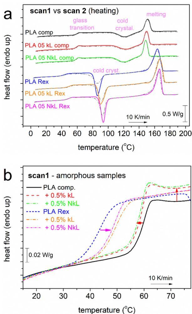
Fig. 3 (a) DSC traces during heating at  $10\text{ K min}^{-1}$ , for all samples shown comparatively for scan 1 (solid-colored lines, initially amorphous) and scan 2 (dash-dotted grey lines). Heat flow is shown upon normalization to the samples' mass. (b) Detailed view of the glass transition step of scan 1 (amorphous systems). The added arrows mark the effects on the temperature position and the  $\Delta C_p$  of glass transition by the addition of kL and NkL.
