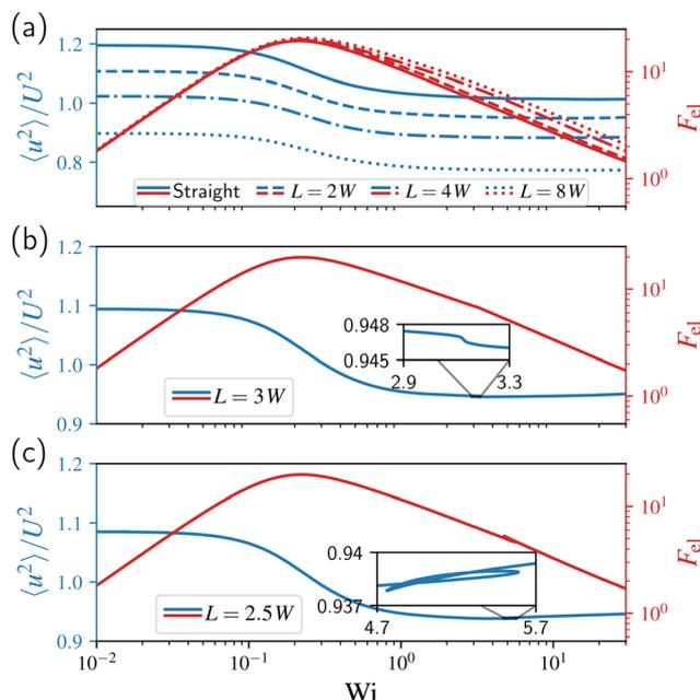
**Fig. 5** Mean squared velocity  $\langle u^2 \rangle / U^2$  and elastic Helmholtz free energy  $F_{el}$  compared to  $Wi$  for (a) a straight channel with a total length  $31W$  as well as concavities of various lengths  $L$ , (b) an expansion-contraction with length  $L = 3W$  showing a potentially supercritical behavior, and (c) an expansion-contraction with length  $L = 2.5W$  showing a subcritical behavior. All concavities have a depth  $D = W$ .
