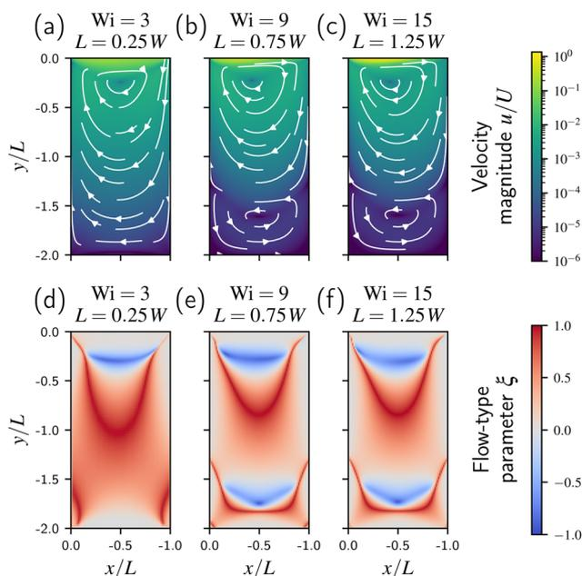
Fig. 12 Cavities of fixed ratio  $D/L = 2$ . Displayed are (a)–(c) the steady-state velocity (using a  $\log_{10}$ -scale) with streamlines and (d)–(f) the flow-type parameter  $\xi$ . The length varies from (a) and (d)  $L = 0.25W$ , to (e) and (f)  $L = 0.75W$ , and finally (c) and (f)  $L = 1.25W$ . We adjust the Weissenberg numbers such that the Deborah number  $De = Wi \cdot W/L = 12$  remains constant.
