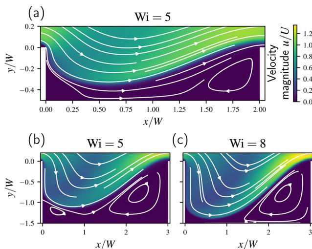
**Fig. 9** Velocity magnitude  $u$  and streamlines for the short expansion-contractions using the steady-state numerical data with (a) depth  $D = 0.5W$  and length  $L = 2W$ ; (b) and (c) depth  $D = 1.5W$  and length  $L = 3W$  at two different Weissenberg numbers. We note the shear localization in (a) which does not align with the boundaries of the vortices, and the extra recirculation inside the concavity in (b) compared to (c).
