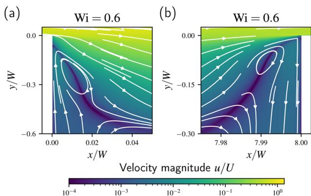
**Fig. 8** Velocity magnitude  $u$  (using a  $\log_{10}$ -scale) and streamlines for the expansion-contraction with  $D = W$  and  $L = 8W$  at  $Wi = 0.5$  focused on (a) the vertical lip vortex at the wall of the expansion phase and (b) the vertical lip vortex at the wall of the contraction phase. These lip vortices are narrow and we emphasize the different scaling in  $x$ - and  $y$ -axis.
