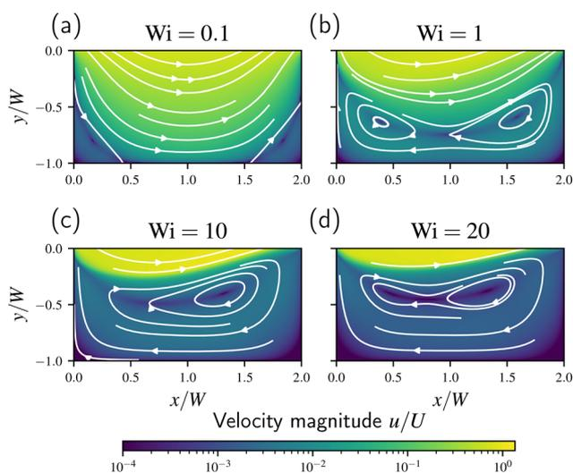
**Fig. 10** Velocity magnitude  $u$  (using a  $\log_{10}$ -scale) and streamlines for a long cavity, where  $D = W$  and  $L = 2W$ , using the steady-state numerical data at (a)  $Wi = 0.1$ , (b)  $Wi = 1$ , (c)  $Wi = 10$ , and (d)  $Wi = 20$ . We note the change from (a) an expansion-contraction towards (c) and (d) a cavity with different number of vortices.
