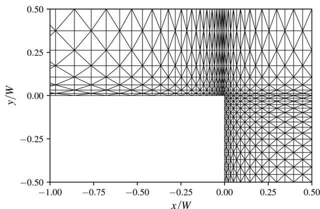
**Fig. 3** Schematic of the mesh around the upstream re-entrant corner illustrating the different densities of the elements ( $D = W, L = W$ ). Shown is a coarse mesh created only for visualization purposes and not for simulations. The total number of elements is 6144 compared to the actual mesh used with 393 216 elements.
