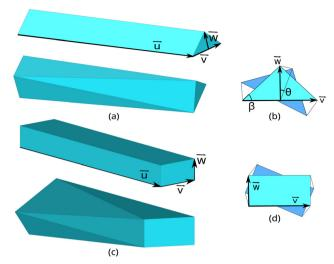
Fig. 1 Sketch of the *n*-prisms. (a) A 3-prism. Side view of an untwisted (above) and a twisted (below) 3-prism with the localized coordinate system visualized. (b) Front and back faces of a 3-prism with twist  $\theta$ . (c) A 4-prism. Side view of an untwisted (above) and a twisted (below) 4-prism with the localized coordinate system visualized. (d) Front and back faces of a twisted 4-prism
