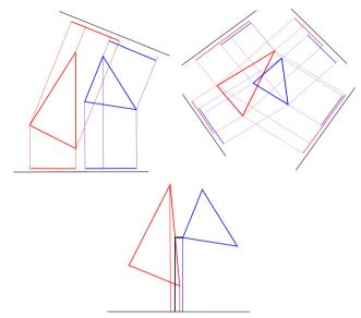
**Fig. 8** Sketch to visualize the separating axes. Top Left: An example of non-overlapping triangles with one separating axis and an unsuccessful attempt shown. Top Right: An example of overlapping triangles with some attempts of finding a separating axis shown. Bottom: An example of the shortest distance modification.
