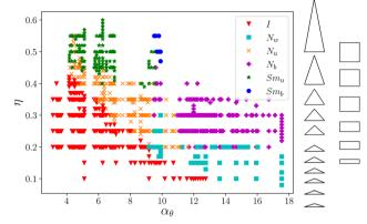
Phase diagrams of both 3-prisms and 4-prisms plotted together as a function of their aspect ratio with a sketch of the size comparison between the particle shapes.
