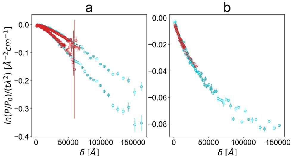
Fig. 7 Data matching of Larmor (red) and Delft (cyan) SESANS data for PS+GO (a, upper) PMMA+GO (a, lower) and PS+GNP (b). The reduced Larmor data exhibit a lower maximum measured spin-echo length  $\delta$  but show good matching and overlap with the Delft data.
