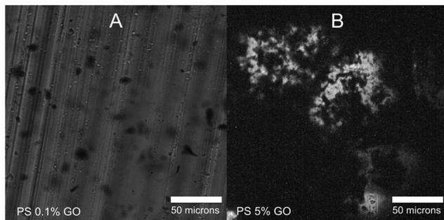
**Fig. 2** Optical microscopy images of pressed PS+GO samples with (A) 0.1% GO for reference, displaying well-dispersed graphene oxide and (B) 5% GO with substantially larger inhomogeneities with diameters on the order of 30–50 microns across. The bright regions in (B) are assumed to be positions on the sample thin enough to allow light transmission.
