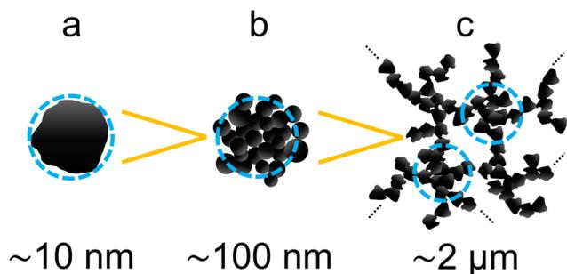
Fig. 5 Illustration of the proposed structural hierarchy for the carbon black nanocomposite. The blue dashed circles indicate the approximate length scale observed in the measurements. The illustrated length scales from left to right are (a) carbon black nanoparticles, (b) carbon black aggregates, and (c) further agglomerate structures. The length scale of the agglomerate structures reflects either their radius of gyration or an average separation within the nanofiller network.
