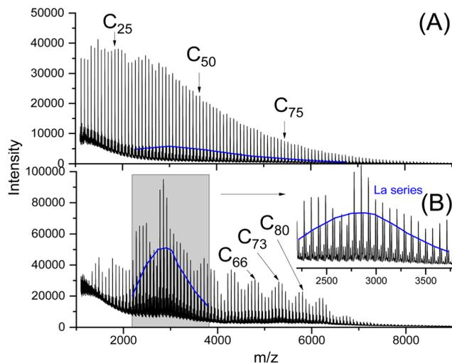
Fig. 4 MALDI TOF mass spectra of cPLA 2B, Table 2, (A) after annealing for 2 d at  $120\text{ }^\circ\text{C}$  (B) after annealing for 28 d at  $140\text{ }^\circ\text{C}$  in the presence of DSTL (Table 3), (La means linear chains with COOH end groups).
