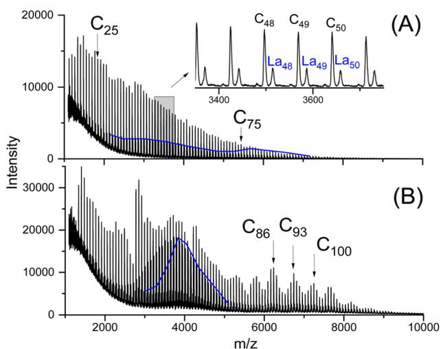
Fig. 3 MALDI TOF mass spectra of cPLA 3B, Table 1 (A) after annealing for 2 d at  $120\text{ }^\circ\text{C}$ , (B) after annealing for 28 d at  $140\text{ }^\circ\text{C}$  in the presence of  $\text{SnOct}_2$  (Table 3), (La means linear chains with COOH end group).
