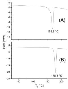
Fig. 6 DSC heating traces (1st heating) of (A) cPLA 3B, Table 3 (annealed at 120  $^{\circ}\text{C/2}$  d, (B) the same PLA after annealing at 140  $^{\circ}\text{C}$  for 28 d.
