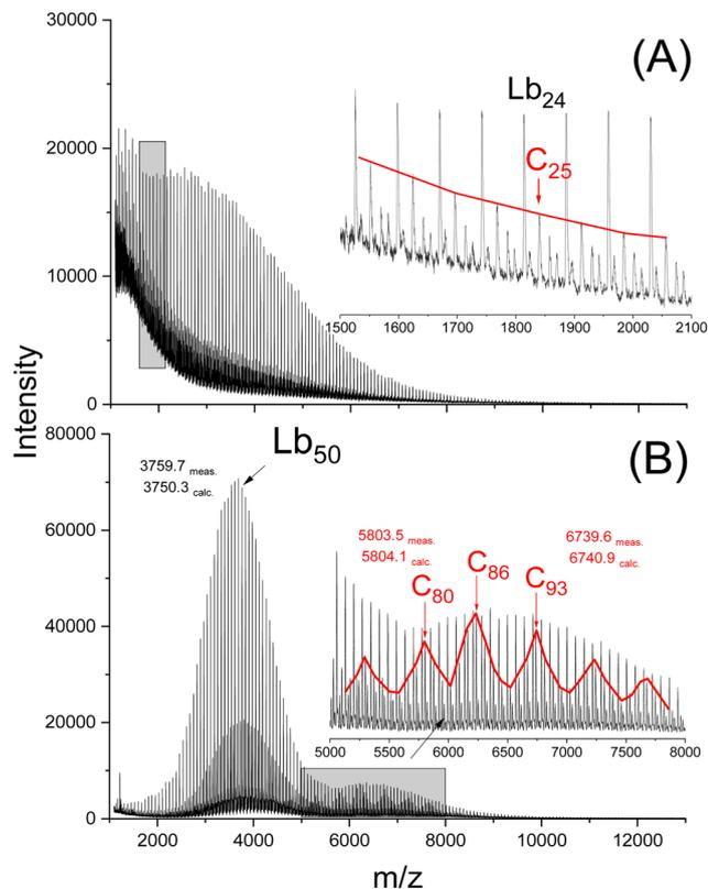
Fig. 5 MALDI of a PLA ethyl ester prepared by ROP of LA initiated with ethyl lactate (LA/In = 100/1) and catalyzed with SnOct<sub>2</sub> (LA/Cat = 400/1) (Table 4): (A) virgin polymerization product after 1 h at 160 °C, (B) after annealing for 28 d at 140 °C, (Lb means linear chains with COOEt end groups).
