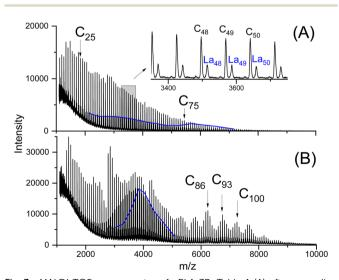
Fig. 3 MALDI TOF mass spectra of cPLA 3B, Table 1 (A) after annealing for 2 d at 120 °C, (B) after annealing for 28 d at 140 °C in the presence of SnOct<sub>2</sub> (Table 3), (La means linear chains with COOH end group)
