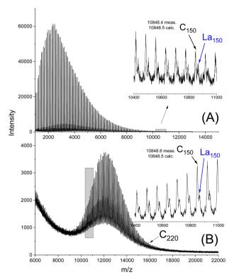
Fig. 1 MALDI TOF mass spectra of the cPLA prepared with LA/Cat 50/1 in 0.5 M solution (3A, Table 1: (A) virgin sample, (B) GPC fraction 11 (La means linear chains with COOH end groups).
