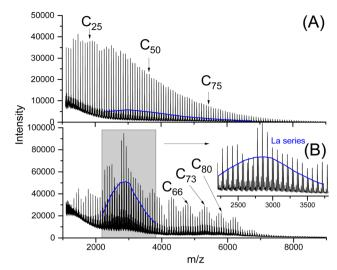
Fig. 4 MALDI TOF mass spectra of cPLA 2B, Table 2, (A) after annealing for 2 d at 120  $^{\circ}$ C (B) after annealing for 28 d at 140  $^{\circ}$ C in the presence of DSTL (Table 3), (La means linear chains with COOH end groups).
