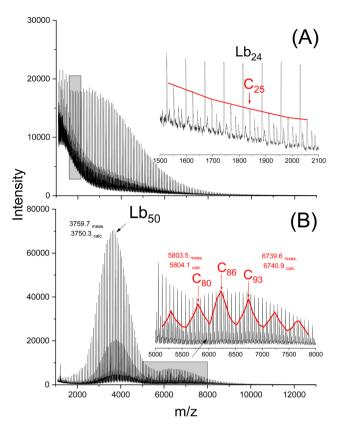
Fig. 5 MALDI of a PLA ethyl ester prepared by ROP of LA initiated with ethyl lactate (LA/In = 100/1) and catalyzed with SnOct<sub>2</sub> (LA/Cat = 400/1) (Table 4): (A) virgin polymerization product after 1 h at 160 °C, (B) after annealing for 28 d at 140 °C, (Lb means linear chains with COOEt end groups)
