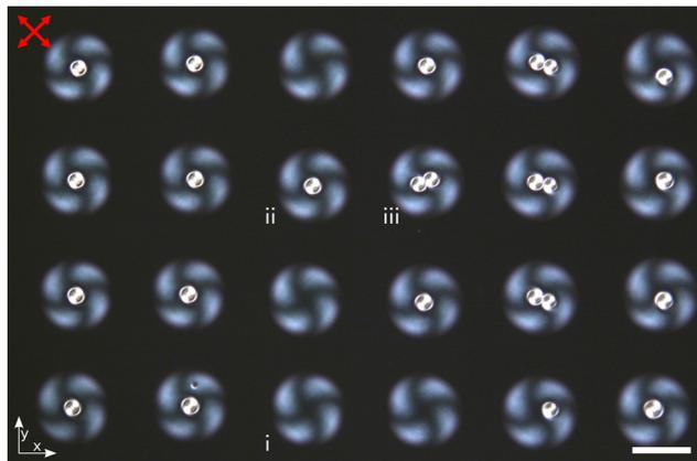
Fig. 4 POM image (experiment) of a grid of 30 droplets of E7 + 0.5 wt% R811 with  $d \sim 100 \mu\text{m}$ . Letters highlight three distinct structures. The axes of the polarisers are at  $\theta = \frac{\pi}{4}$  and  $\theta = \frac{3\pi}{4}$  to the vertical, as shown by the red double-headed arrows. Scalebar:  $100 \mu\text{m}$ . Image taken at  $20^\circ\text{C}$ . At this temperature, the pitch of E7 + 0.5 wt% R811 is  $20 \mu\text{m}$ , giving  $N_1 = 1.16$ .
