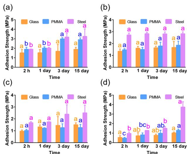
Fig. 3 Time-dependent adhesion strengths of poly[TA-MoS<sub>2</sub>] under water. (a) TA : MoS<sub>2</sub> = 1 : 1; (b) TA : MoS<sub>2</sub> = 5 : 1; (c) TA : MoS<sub>2</sub> = 10 : 1; (d) TA : MoS<sub>2</sub> = 100 : 1. Different letters signify significant differences at  $p < 0.05$ .
