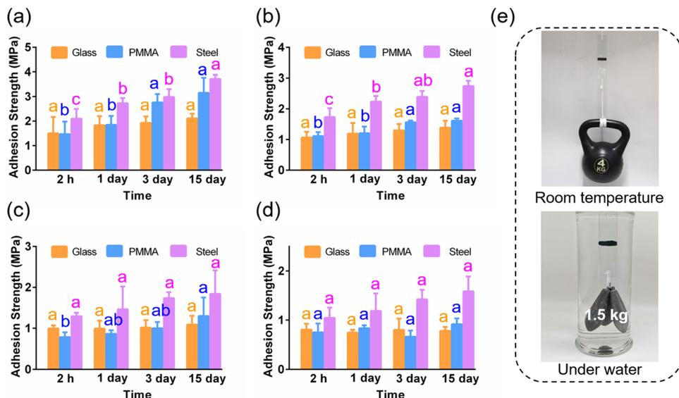
Fig. 2 Time-dependent adhesion strengths of poly[TA-MoS<sub>2</sub>]. (a) TA : MoS<sub>2</sub> = 1 : 1; (b) TA : MoS<sub>2</sub> = 5 : 1; (c) TA : MoS<sub>2</sub> = 10 : 1; (d) TA : MoS<sub>2</sub> = 100 : 1; (e) macroscopic adhesion behavior of poly[TA-MoS<sub>2</sub>]. Different letters signify significant differences at  $p < 0.05$ .
