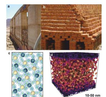
Fig. 17 Earth construction materials, examples, and scientific questions: (a) rammed earth constructions, (b) rural brick kiln, (c) water-ion structures from semiatomistic simulations of Ca ions solutions confined between charged surfaces, 364 and (d) mesoscale porous structures of cement hydrate gels from coarse-grained simulations, where particle sizes are on the order of 10-50 nm. 365
