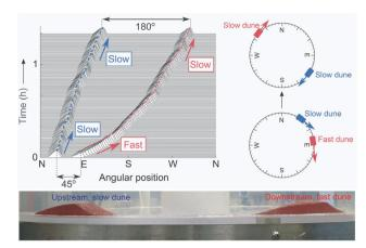
Two equal-size miniature dunes are initially placed 45° apart in a periodic annular channel. Due to drag imposed by the water current, they start migrating and drift apart, and converge over long times to a symmetric antipodal configuration 180° apart. 333
