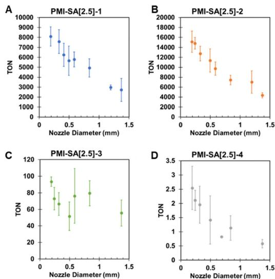
Fig. 3 TON values for PMI-SA[2.5] extruded from different nozzle diameters with gels containing catalysts **1** (A) **2** (B) **3** (C) and **4** (D) exposed to light for 18 hours (nozzle diameters used ranged from 0.2 mm to 1.37 mm).
