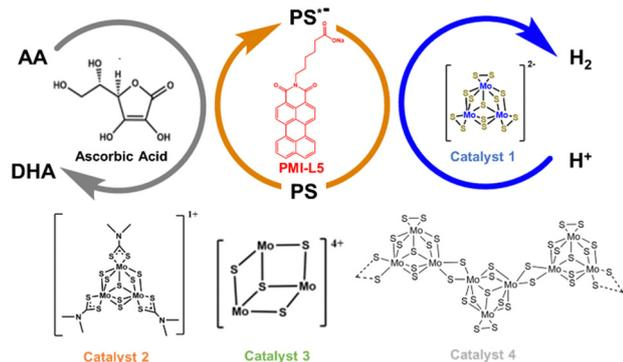
**Scheme 1** Proposed mechanism of HER photocatalysis using PMI as a photosensitizer (PS) and ascorbic acid (AA) as a sacrificial electron donor. Electron transfer from AA to PMI produces dehydroascorbic acid (DHA) which can parasitize electron transfer from AA (catalyst structures are also shown).
