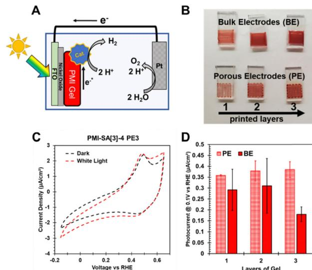
**Fig. 6** (A) Schematic diagram of the photoelectrocatalysis setup used in experiments. (B) photograph of the non-porous bulk electrodes (BE) and porous electrodes (PE) printed with thicknesses of 1, 2, or 3 layers. (C) CV of a single layer of PMI-SA[3]-4 printed on FTO-NiO under both dark and illuminated conditions. (D) Values of the measured photocurrent at +0.1 V vs. RHE for PMI-SA[3]-4 of printed BE and PE with 1 to 3 layers.
