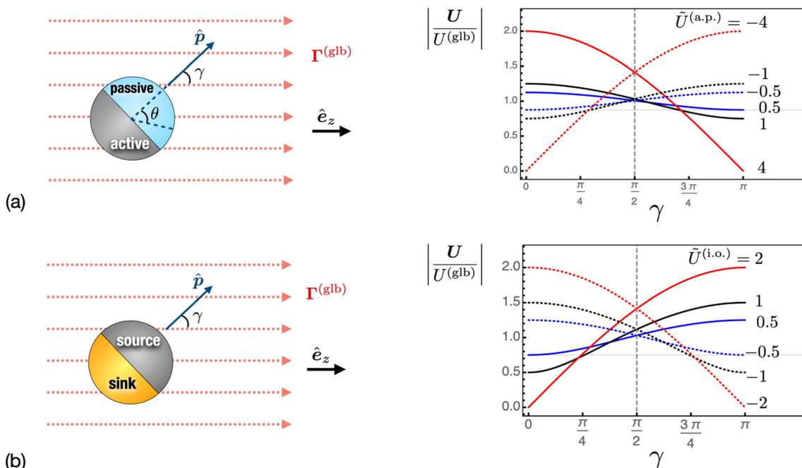
Fig. 2 Two self-phoretic Janus models of (a) active-passive (a.p.) and (b) sink-source (i.o.) composition are undergoing globally-driven phoresis by the far-field flux  $\Gamma^{(\text{glb})}$ . The angle  $\gamma$  defines the orientation of the Janus director  $\hat{p}$  with respect to  $\Gamma^{(\text{glb})}$ . Solid lines represent positive values of  $\tilde{U}^{(\text{a})}$ , while dashed lines represent negative values.
