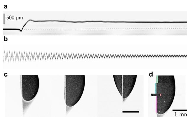
Fig. 9 Force microscopic measurement conducted on a confocal microscope. Here, 10  $\mu\text{l}$  water drops slide on SOCAL surfaces (*cf.* Fig. 6c). (a) Kymograph of the blade deflection upon drop contact, measured with the reflection channel of an *xt*-scan. (b) Calibration curve to determine the spring constant of the blade, here approx.  $0.21 \text{ N m}^{-1}$ . (c) Atto-dyed, steady-state drop footprints, and faintly the probing metal blade. (d) Overlay of various relaxed drop footprints.
