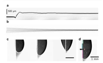
Fig. 9 Force microscopic measurement conducted on a confocal microscope. Here, 10 µl water drops slide on SOCAL surfaces (cf. Fig. 6c). (a) Kymograph of the blade deflection upon drop contact, measured with the reflection channel of an xt-scan. (b) Calibration curve to determine the spring constant of the blade, here approx.  $0.21 \text{ N m}^{-1}$ . (c) Atto-dyed, steady-state drop footprints, and faintly the probing metal blade. (d) overlay of various relaxed drop footprints.
