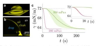
Fig. 4 Sessile drop on lubricated surface, cloaked by PDMS oil. (a) Threedimensional view of PDMS oil on the drop, obtained by laser scanning confocal microscopy. (b) Side view of the angular averaged 3D stack. Images adapted from ref. 89 (c) temporal evolution of pendant drop on PDMS elastomer with swollen with 200 mPa s (red) and 350 mPa s (green) PDMS oil. The shaded region shows the standard deviation of experimental repeats. Data adapted from ref. 207.
