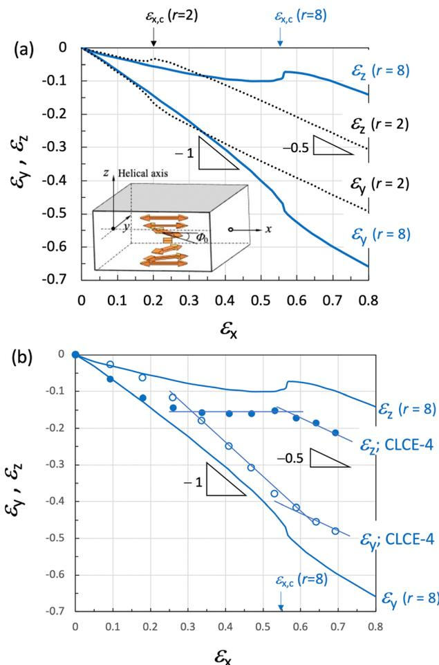
Fig. 9 (a) Initial director angle  $\Phi_0$  of a cholesteric helix in the model. Lateral true strains  $\varepsilon_y$  and  $\varepsilon_z$  as a function of longitudinal true strain  $\varepsilon_x$  calculated for  $r = 8$  and 2. The critical strain is  $\varepsilon_{x,c} \approx 0.55$  ( $\lambda_c \approx 1.73$ ) or 0.20 ( $\lambda_c \approx 1.20$ ) for  $r = 8$  or 2, respectively. (b) Comparison of the model prediction with  $r = 8$  with the data of CLCE-4 reproduced from Fig. 6b.
