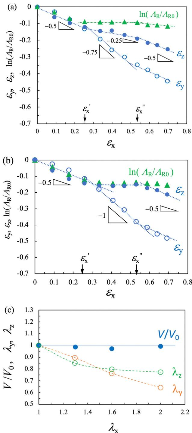
Fig. 6 Lateral true strain in  $y$ ,  $z$ -direction ( $\epsilon_y$  and  $\epsilon_z$ ), and  $\ln(A_R/A_{R0})$  as a function of longitudinal true strain in  $x$ -direction ( $\epsilon_x$ ) for (a) CLCE-0 and (b) CLCE-4. (c) Changes in dimensions in the  $y$ - and  $z$ -directions ( $\lambda_y$  and  $\lambda_z$ ) and relative volume ( $V/V_0$ ) as a function of stretch in the  $x$ -direction ( $\lambda_x$ ) for CLCE-0. The dashed lines are guides for eyes.
