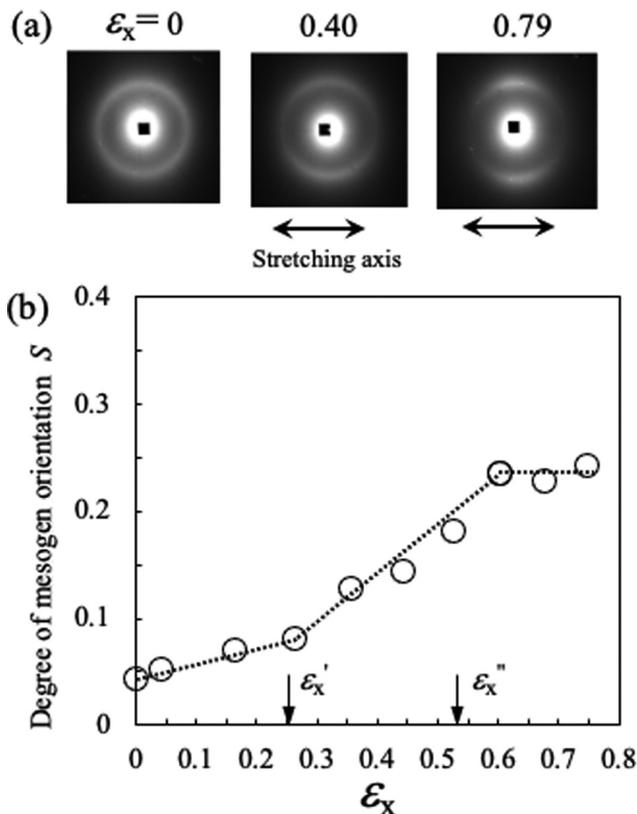
Fig. 5 (a) Two dimensional wide-angle X-ray scattering patterns for CLCE-0 at various  $\epsilon_x$  values. (b) Degree of orientation of local directors in the elongation ( $x$ ) direction as a function of tensile true strain in the  $x$ -direction ( $\epsilon_x$ ) for CLCE-0.
