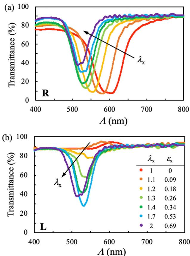
Fig. 3 Transmission spectra of CLCE-4 under uniaxial extension for (a) right- and (b) left-handed circularly polarized incident light as a function of stretch ( $\lambda_x$ ) or true strain ( $\epsilon_x$ ) in the  $x$ -direction.
