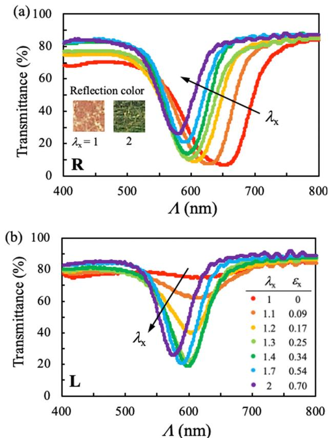
Fig. 2 Transmission spectra of CLCE-0 under uniaxial extension for (a) right- and (b) left-handed circularly polarized incident light as a function of stretch ( $\lambda_x$ ) or true strain ( $\epsilon_x$ ) in the  $x$ -direction. The insets in (a) display the change in reflection color after the stretching of  $\lambda_x = 2$ .
