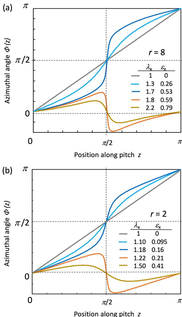
Fig. 10 Director angle  $\phi$  as a function of position along pitch  $z$  at various degrees of longitudinal true strain ( $\epsilon_x$ ) calculated for (a)  $r = 8$  and (b)  $r = 2$ . The critical strain is  $\epsilon_{x,c} \approx 0.55$  ( $\lambda_{x,c} \approx 1.73$ ) or 0.20 ( $\lambda_{x,c} \approx 1.20$ ) for  $r = 8$  and 2, respectively.
