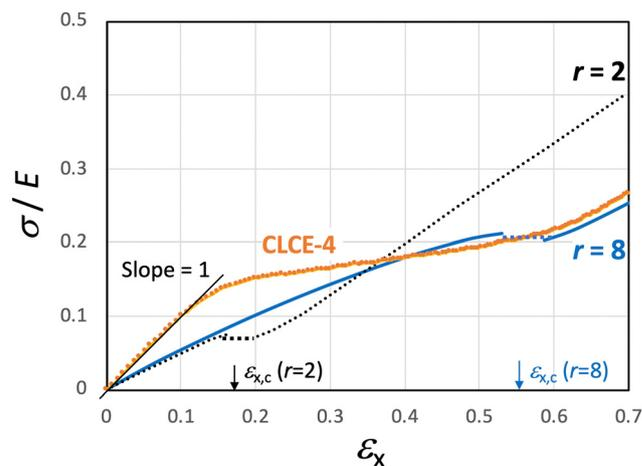
Fig. 11 Nominal tensile stress ( $\sigma$ ) reduced by Young's modulus ( $E$ ) as a function of longitudinal true strain ( $\epsilon_x$ ) calculated for  $r = 8$  and 2. The critical strain  $\epsilon_{x,c} \approx 0.55$  ( $\lambda_{x,c} \approx 1.73$ ) and 0.20 ( $\lambda_{x,c} \approx 1.20$ ) for  $r = 8$  and 2, respectively. The data of CLCE-4 are reproduced from Fig. 7.
