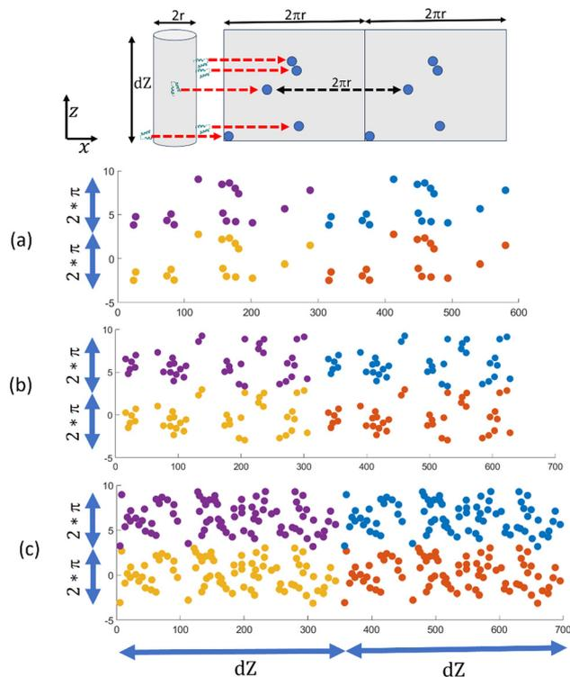
Fig. 3 Top panel shows the cylinder (radius  $r$ ) to plane (width  $2\pi r$ ) mapping. Red arrows indicate new positions of Z33s in the mapped plane. Mapped distribution is repeated twice in radial direction for periodicity. (a)–(c) show the mapped distribution for ligand-filler ratio of 1/25, 1/10 and 1/5 respectively. Four color indicates 4 periodic distributions.
