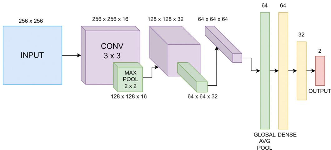
Fig. 1 Example sequential CNN architecture, including layer output dimensions. "CONV" represents a  $3 \times 3$  convolutional layer and "MAX POOL" and "GLOBAL AVG POOL" maximum and global average pooling.
