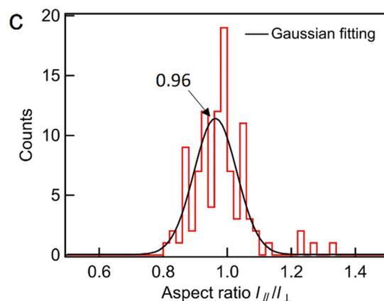
**Fig. 5** (a) Definition of the aspect ratio of the BPI crystal. (b) Relationship between the aspect ratio and the crystal size and (c) dispersion of the aspect ratio of a 5  $\mu\text{m}$  thick rubbing cell.
