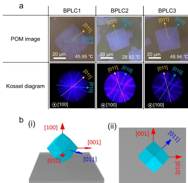
Fig. 2 (a) POM images of BPI crystal and the corresponding Kossel diagrams. (b) Schematic of BPI crystal geometry in (i) perspective and (ii) top views.
