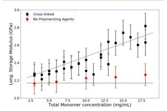
Fig. 4 Longitudinal storage modulus versus total monomer concentration (7) for PA gels of crosslinker concentration (C) = 3.33% fully polymerized and cross-linked (black) and monomer solutions (red). Guide lines added for clarity.
