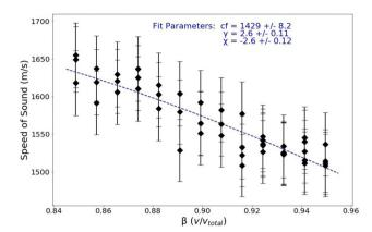
Fig. 7 The speed of sound of the hydrogel *versus* the volumetric water fraction within the sample. The poroelastic wave speed fit for PA gels in the intermediate hydration regime is indicated with a dashed line. Fit parameters are listed.
