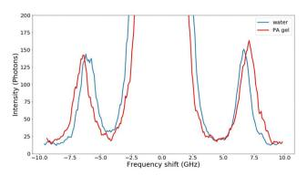
Fig. 1 Two Brillouin spectra. The blue curve is that of water and the red curve is that of a polyacrylamide hydrogel. The Brillouin shift,  $\Omega$ , is the position of the two peaks. The central peak (extending upward out of the graph) results from elastic scattering.
