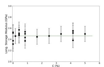
Fig. 5 Longitudinal storage modulus *versus* crosslink density for PA gels of total monomer concentration (T) = 12%. Guide line added for clarity.
