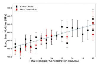
Loss modulus *versus T* for PA gels of C = 3.33% (black) and C = 0%Fig. 9 (red). Guide line added for clarity
