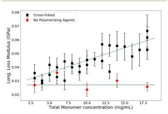
Fig. 8 Loss modulus versus T for PA gels of C = 3.33% (black) and monomer solutions (red). Guide lines added for clarity
