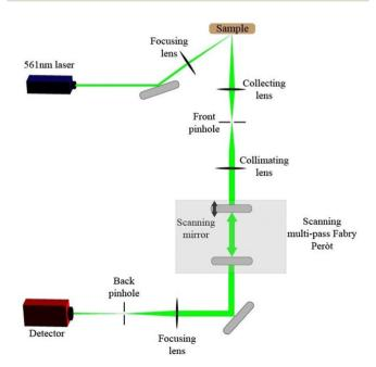
Fig. 2 A schematic representation of our Brillouin spectrometer.
