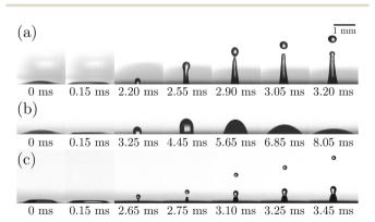
Fig. 4 High-speed images of jetting following bubble bursting at the surface of a (a) pure NaCl solution, (b)  $0.05~{\rm g~L^{-1}}$  BSA solution, and (c)  $0.05 \,\mathrm{g}\,\mathrm{L}^{-1}\,\mathrm{BSA} + 0.1 \,\mathrm{g}\,\mathrm{L}^{-1}\,\mathrm{Tween}$  80 solution. The aging time of the bubble is controlled to be  $t_a = 300$  s. The origin of time at 0 ms represents the start of bubble cap rupture
