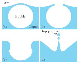
Fig. 1 Schematics of jet drop ejection by bubble bursting: (a) bubble cap film drainage at the free surface; (b) cap film rupture; (c) cavity collapse; and (d) jet ejection and jet drop detachment.
