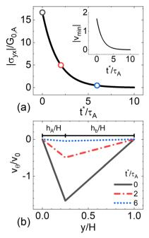
Fig. 7 Relaxation of normalized (a) shear stress and (b) velocity profiles at three times (O in (a)) during flow cessation. Flow achieved steady state before flow was stopped;  $v_0$  is the imposed wall velocity during the preceding shear. Time is normalized by the relaxation time of fluid A,  $\tau_A$ ;  $t^* = t - t_c$  denotes the elapsed time after flow ceases. (a, inset) Shear stress and  $|v_{min}|$  decay with the same time constant.
