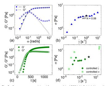
Fig. 2 Frequency sweep (a) and flow curve (b) of P234-NaF. (a) A Maxwell model fit (solid and dashed lines) yields estimates of  $G_0$  = 3.7  $\pm$  0.3 Pa and  $\tau$  = 9.1  $\pm$  0.4 s. (b) Shear banding is expected in the flow curve plateau region ( $\dot{\gamma} \approx 0.2-2 \text{ s}^{-1}$ , N = 0.06). An SAOS aging test (c) and flow curve (d) of P234-NaCl. On each flow curve. \* denotes the shear rate investigated in shear startup and cessation of flow
