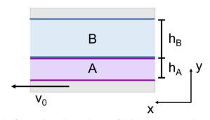
Fig. 1 Couette flow of two adjacent UCM fluids between parallel plates. The two fluid volumes are segregated perpendicular to the flow direction, with fluid A near the lower plate (y = 0) and fluid B near the upper plate  $(y = h_A + h_B = H)$
