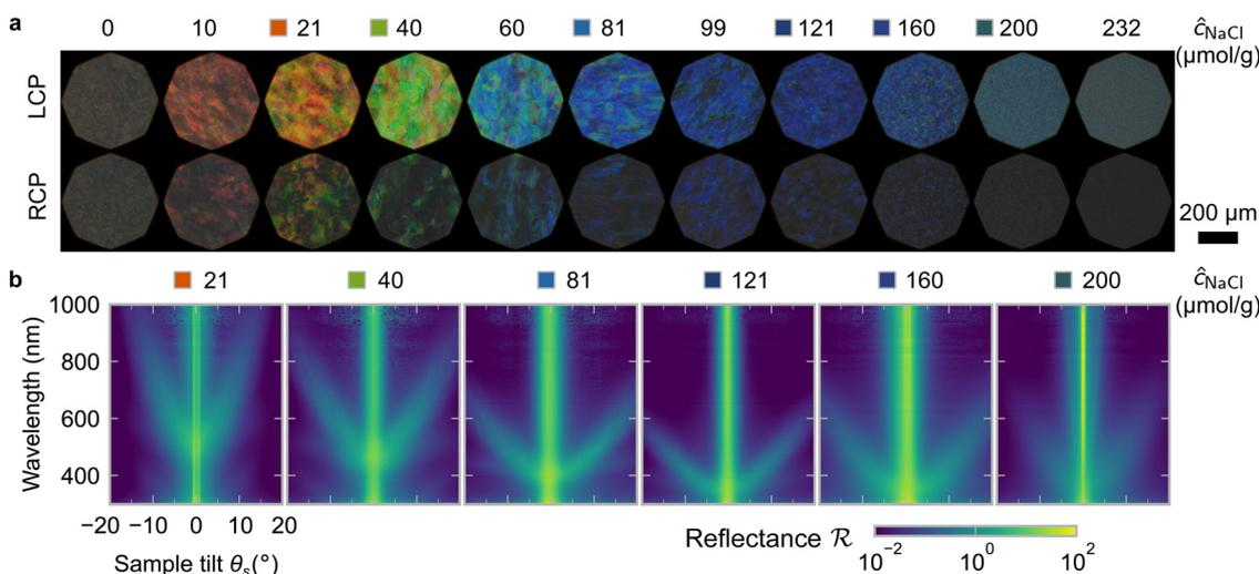
Fig. 3 (a) Polarised optical microscopy (POM) in reflection mode for photonic CNC films with increasing NaCl:CNC ratio  $\hat{c}_{\text{NaCl}}$ . Images were acquired through a left- and right-circularly polarised analyser (LCP and RCP respectively). (b) Tilt scan data for selected  $\hat{c}_{\text{NaCl}}$  values. Colour bar indicates log-scale reflectance  $\mathcal{R}$  normalised to a diffuse reflectance standard.
