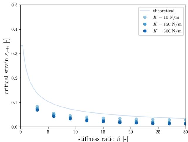
Fig. 3 Critical strain  $\varepsilon = 1 - 1/\sqrt{\beta_g}$  vs. cortical–subcortical stiffness ratio. Theoretical results are taken from Holland *et al.*<sup>66</sup>
