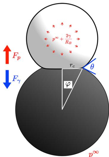
Fig. 9 Sketch of a more realistic geometry of bubble growth in which the bubble forms a spherical cap on the colloid. The contact angle  $\theta$  and coverage angle  $\phi$  are exaggerated for illustrative purposes. An internal pressure detachment force  $F_p$  and a contact line adhesion force  $F_\gamma$  compete in attaching the bubble to the colloid.
