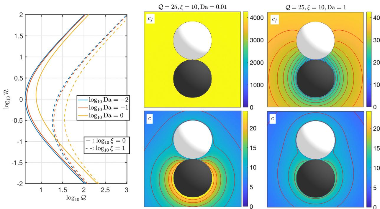
**Fig. 8** Effect of the Damköhler number  $\text{Da}$  on the bubble growth dynamics. Left: Dashed and dash-dotted lines indicate theoretical estimates for  $R_{\text{max}}$  (stable) and  $R_{\text{min}}$  (unstable) respectively. The effect of a non-zero Damköhler number is approximately a shift of the nullclines towards larger values of flux  $\mathcal{Q}$ . Right: Illustration of the fuel (top) and solute (bottom) concentration fields for small and large  $\text{Da}$ .
