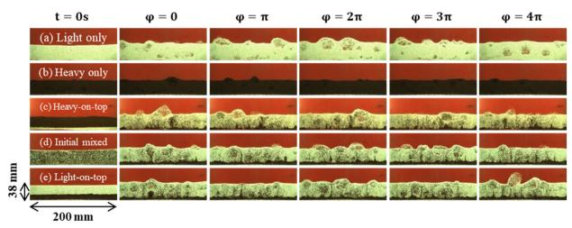
Fig. 7 Time series of front-lit images of experimental cases with only gas flow over the equivalent duration of two vibration periods after statistical steady state is reached for different initial particle configurations (a)-(e).
