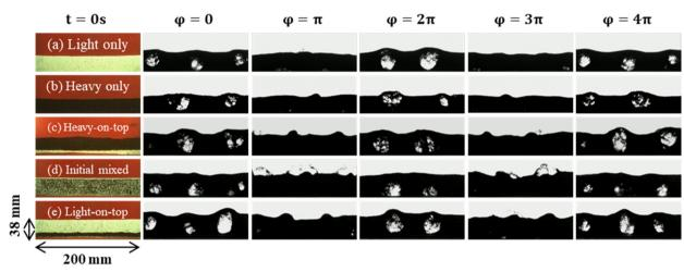
Fig. 3 Time series of backlit images of experimental cases with combined gas flow and vibration over the course of two vibration periods after statistical steady-state is reached for different initial particle configurations (a)-(e).
