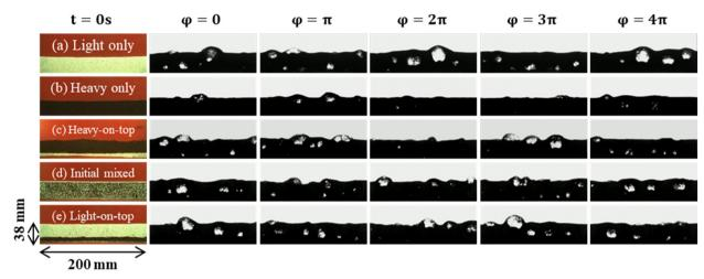
Fig. 6 Time series of backlit images of experimental cases with only gas flow over the equivalent duration of two vibration periods after statistical steady-state is reached for different initial particle configurations (a)-(e).
