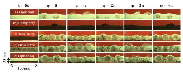
Fig. 4 Time series of front-lit images of experimental cases with combined gas flow and vibration over the course of two vibration periods after statistical steady state is reached for different initial particle configurations (a)-(e).
