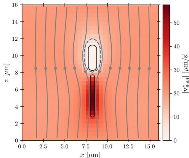
Fig. 4 Cross-section through the dipolar flow field generated by a swimming bacterium, in the cell's moving frame of reference. The image shows the same flow field as in Fig. 2, but in the comoving frame. The cell is swimming in the +z direction. The blue dashed line marks  $Pe_{\text{phage}}^* = 1$ .
