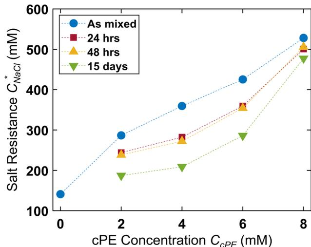
Fig. 6 The temporal evolution of the salt resistance  $C_{\text{NaCl}}^*$  for complex coacervate dispersions.  $C_{\text{NaCl}}^*$ , corresponding to the maximum salt concentration at which dispersions retained turbidity of  $4 \text{ cm}^{-1}$  irrespective of the PE concentration, is shown as a function of comb polyelectrolyte concentration.  $C_{\text{NaCl}}^*$  of the complex coacervate dispersions increases with increasing cPE concentration and is maintained for up to 15 days.
