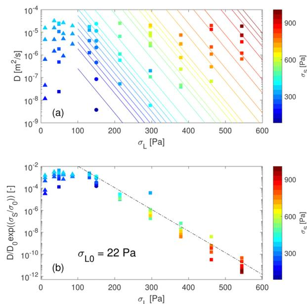
**Fig. 3** (a) All  $D$  obtained for all  $\sigma_{L,S}$  measured shown versus confinement stress. Symbols indicate experiments NL ( $\circ$ ), FL ( $\Delta$ ) and GL ( $\square$ ). Solid lines indicate the trend as described in eqn (1) (b) rescaled data. The dashed line indicates the exponential decay with confinement stress; the stress scale  $\sigma_{L0}$  is indicated in the panel.
