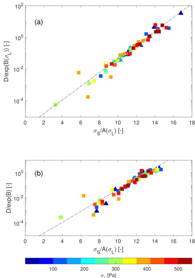
Fig. 5 (a) Rescaled data, dividing out the  $\sigma_L$  dependence for the freely fitted eqn (2), providing  $\sigma_L$ -dependent  $A$  and  $B$ . (b) Rescaled data, now with the fixed  $B = -11.2$  while fitting  $A(\sigma_L)$  as shown as blue squares in Fig. 4(b). The colorbar applies to both panels. The dashed line indicates the exponential intruder stress dependence  $D_0 \exp(\sigma_S)$  in both panels.
