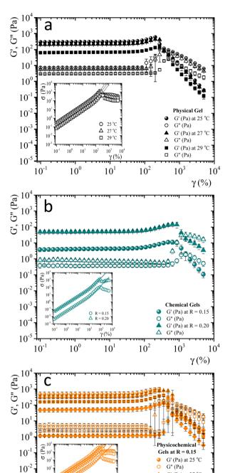
$\gamma$  (%) Fig. 3 Elastic and loss modulus for 5 wt% matured gelatin gels vs.  $\gamma$  at a constant frequency ( $\omega = 1 \text{ s}^{-1}$ ). (a) Matured physical gels at  $T = 25 \,^{\circ}\text{C}$ , 27  $^{\circ}\text{C}$ , and 29 °C. (b) Matured chemical gels at 35 °C for R = 0.15 and R = 0.20. (c) Matured physicochemical gels with R = 0.15 at T = 25 °C, 27 °C, 29 °C, and 30 °C. Insets,  $\sigma$  vs.  $\gamma$ , and the fittings to the BST model (continuous line).
