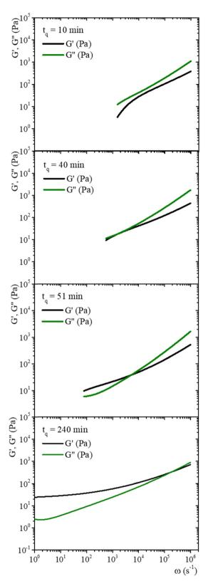
Fig. 8 Time evolution of viscoelastic spectra for gelatin solution after a temperature quench from 35 °C to 25 °C to produce a physical gel measured from  $t_q$  = 10 min to  $t_q \sim 240$  min passing through the gel point.
