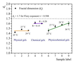
Fig. 4 Fractal dimension for different matured gels aged over four hours.
