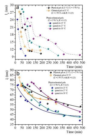
Fig. 10 Characteristic mesoscopic scales as time elapses after the gelation process has started for physical, chemical, and physicochemical gels. (a)  $l_p$  vs. time; dashed lines are a guide to the eye. (b)  $\xi$  vs. time; lines correspond to exponential decay fits.
