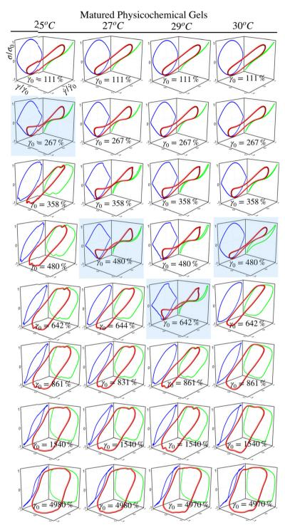
Fig. 6 Normalized 3D Lissajous – Bowditch curves and their projections (elastic representation:  $\sigma/\sigma_0$  vs.  $\gamma/\gamma_0$  or viscous representation:  $\sigma/\sigma_0$  vs.  $\gamma/\gamma_0$ ) for matured physicochemical gels for different  $\gamma_0$ , aged at 25 °C, 27 °C, 29 °C, and 30 °C from a solution with C=5 wt% and R=0.15. Blue shadow corresponds to an imposed strain deformation  $\gamma_0 = \gamma_{\text{break}}$
